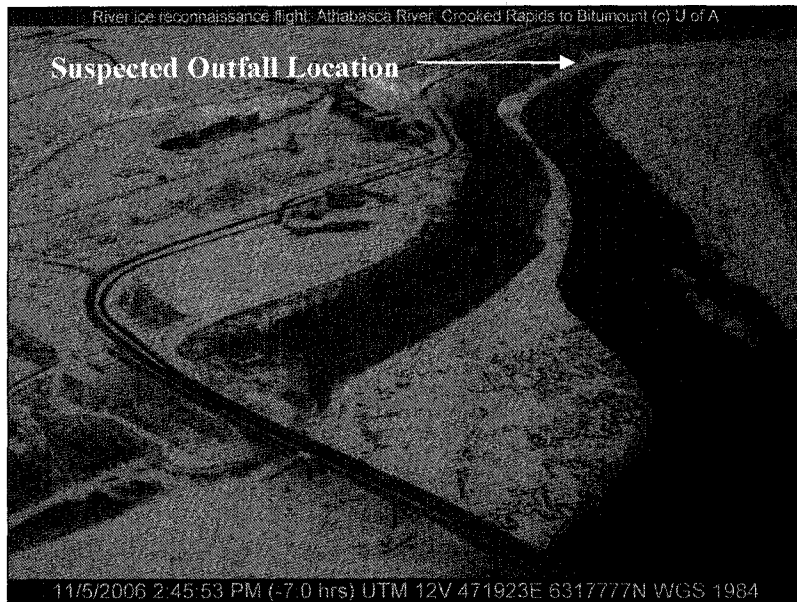
Figure 2.38 Open lead resulting from a warm water outfall near the Suncor Bridge, as seen on November 5, 2006.
