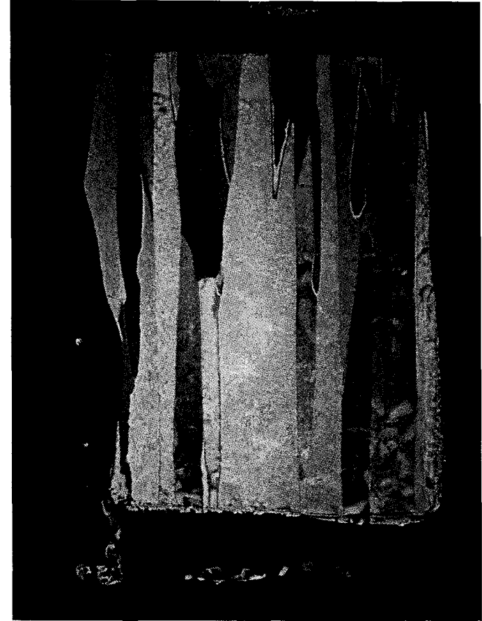
Typical crystal structure of thermal ice cover photographed under polarized light. (Photo courtesy of Karen van Steenis)
