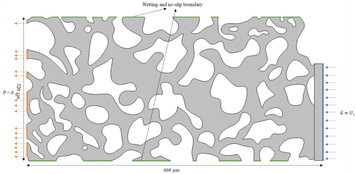
Figure 4.5. Schematic of the complex porous medium and related boundary conditions (white area – solid grains; grey area – pore space).
