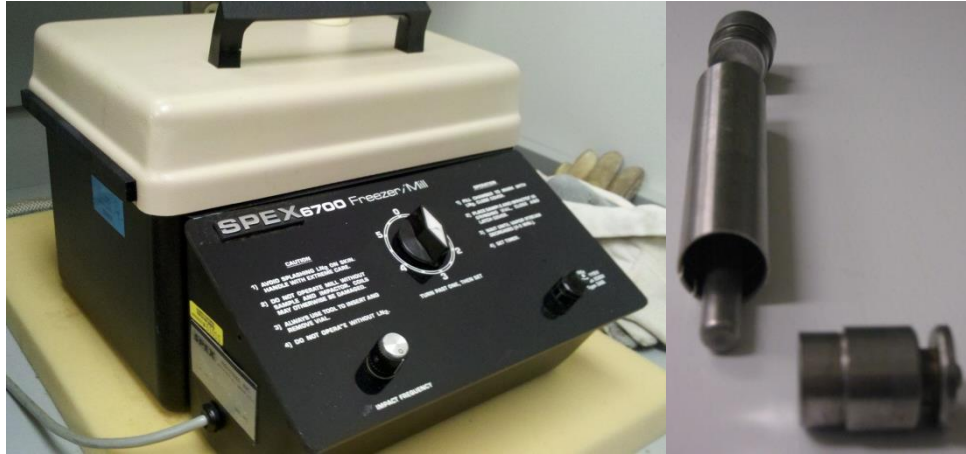
Figure 3.13 Freezer Mill (left) and sample tube with rod (right).
