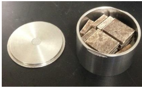
Figure 3.12 Sample chamber filled with square biocomposite specimens
