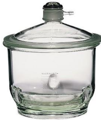
Figure 3.24 Glass vacuum chamber where salt solution filled the bottom of the container to produce a high humidity environment of 97.3%. Image from [20].
