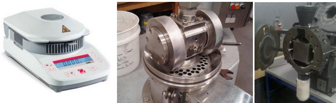
Figure 3.3 Equipment involved with natural fiber pelletization from left to right: Ohaus Moisture Analyzer[1], Amandus Kahl Die Face Mill with Rollers, and Wiley Mill.
