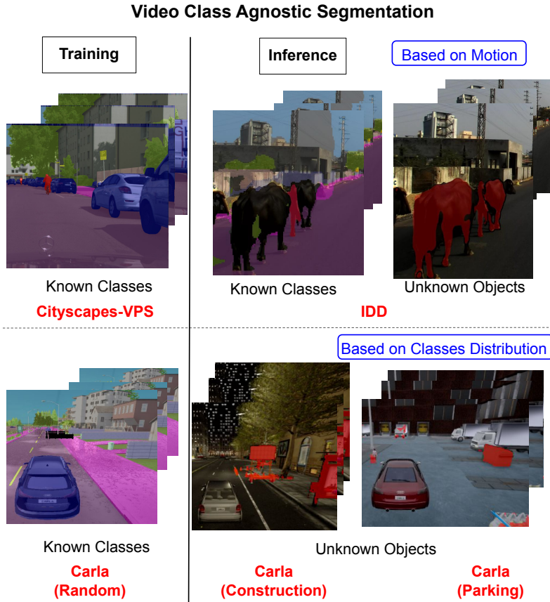
Figure 5.1: Video Class Agnostic Segmentation allows to identify objects outside the closed set of known classes.
