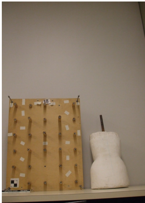
Figure 3.9 (b) Pegboard image from bottom camera using BCA 35° CD 100cm and OD 235cm
