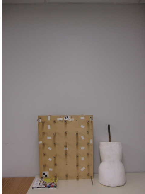
Figure 3.9 (a) Pegboard image from top camera using TCA 35° CD 100cm and OD 235cm
