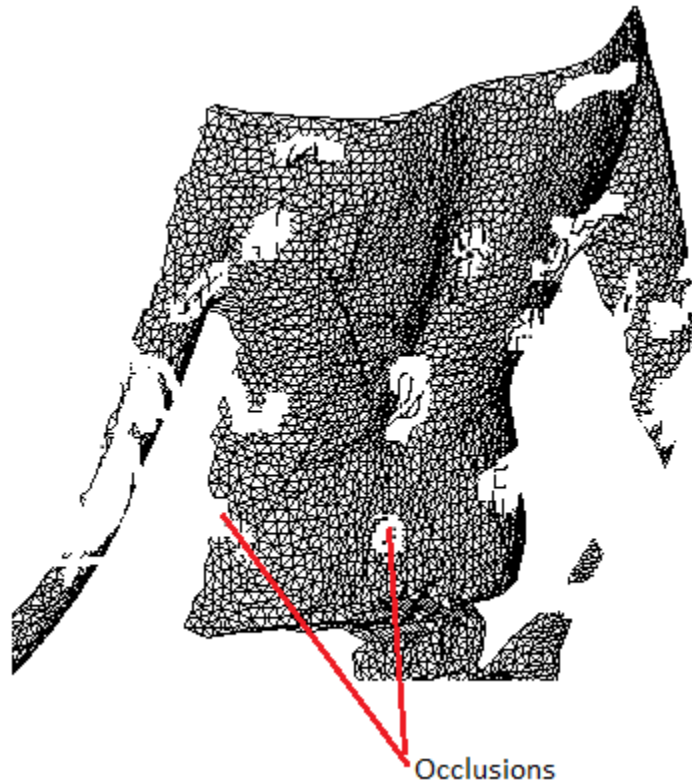
Figure 5.3: Removal of Stray Data Points from Triangulated 3D Point Map
