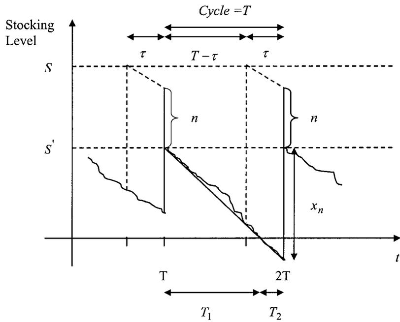
Figure 4.2: Shortage of spare parts during a cycle
