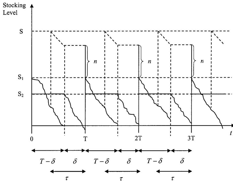
Figure 4.5: Stocking level behaviors according to  $(T, \delta, S)$  control strategy with a procurement lead time of  $\tau \geq \delta$
