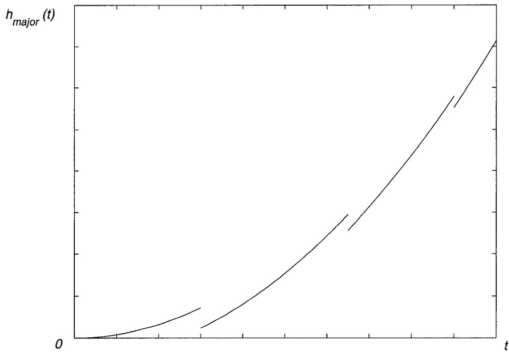
Figure 3.2: The effects of a major failure repair on the major failure rate function
