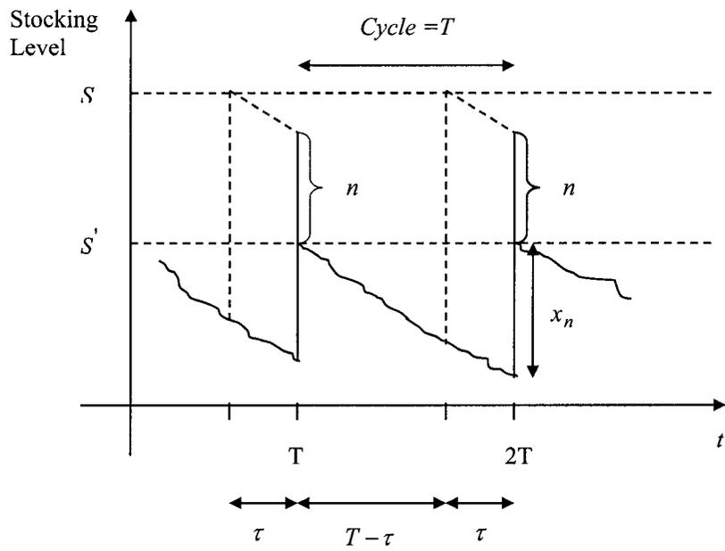
Figure 4.1: Excess of spare parts during a cycle
