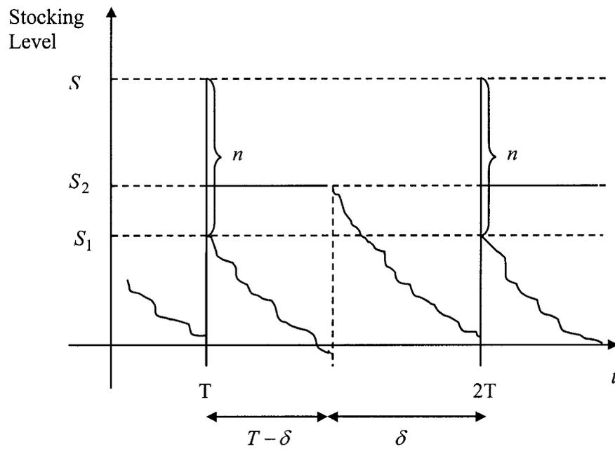
Figure 4.10: Stocking level behavior in a hybrid spare parts model ( $S_1 \leq S_2$ )
