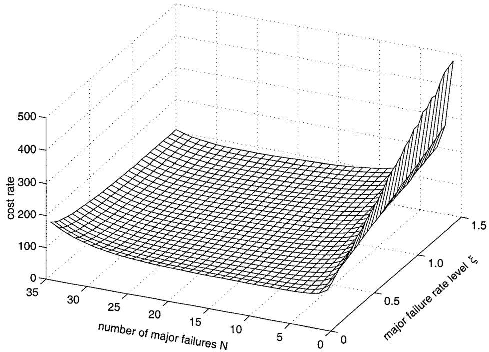
Figure 3.4: Cost rate against the number of major failures and the major failure rate level
