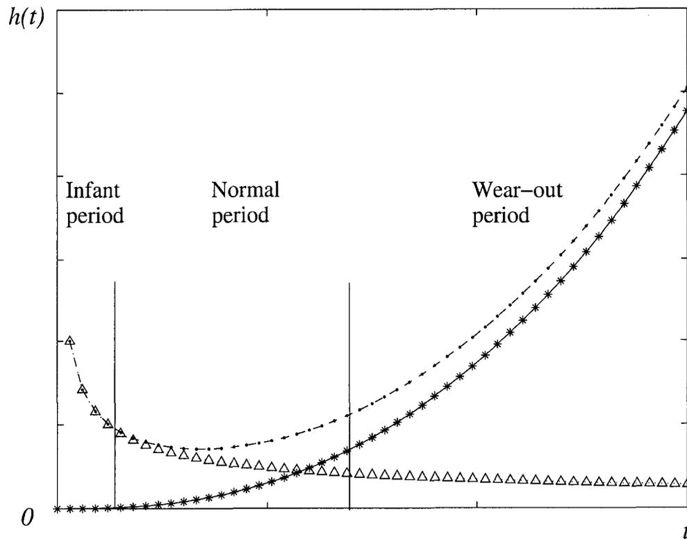
Figure 3.1: The bathtub-shaped failure rate (the point line) as a sum of the major failure rate (the star line) and the minor failure rate (the triangle line)
