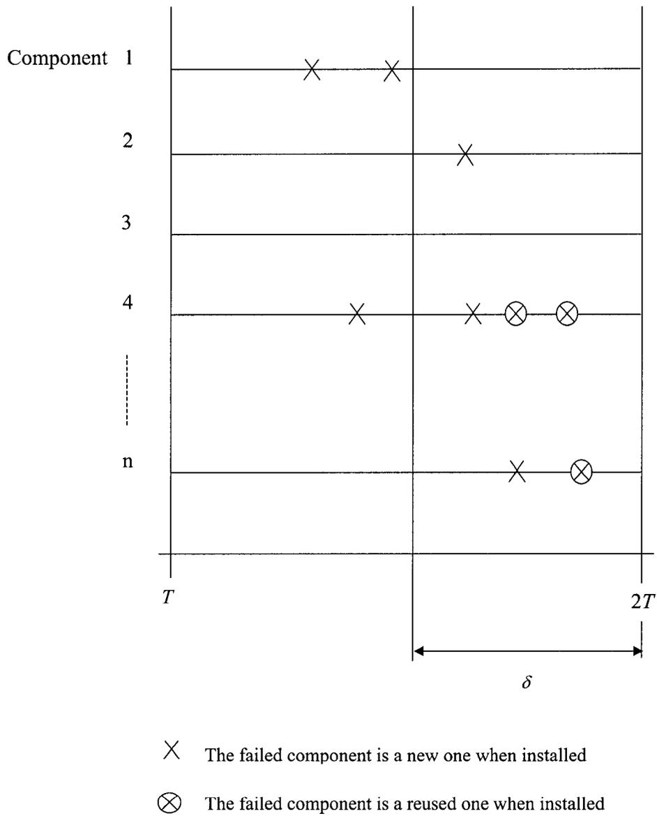
Figure 4.7: Replacement of failed components during one BR interval, with regard to used spare parts
