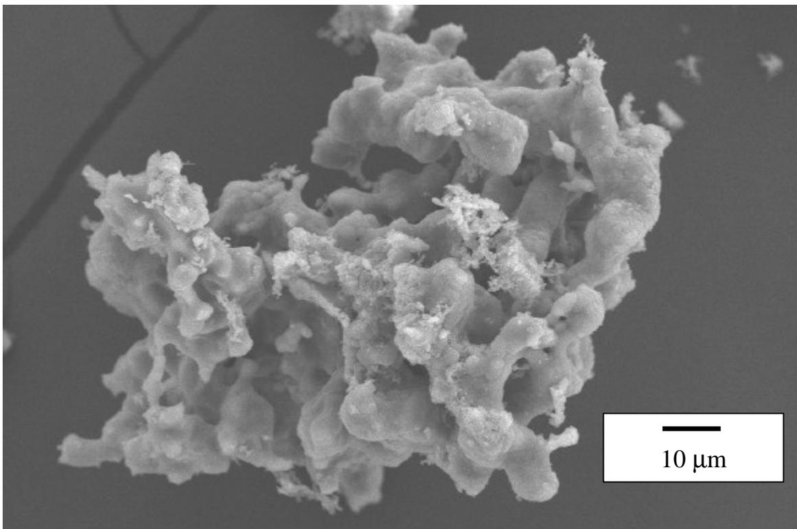
Figure A9. Example of a combustion product from the wood waste burner ash, Primary elements - Ca, with trace Si, Fe, Al, Mg, Cu, Zn
