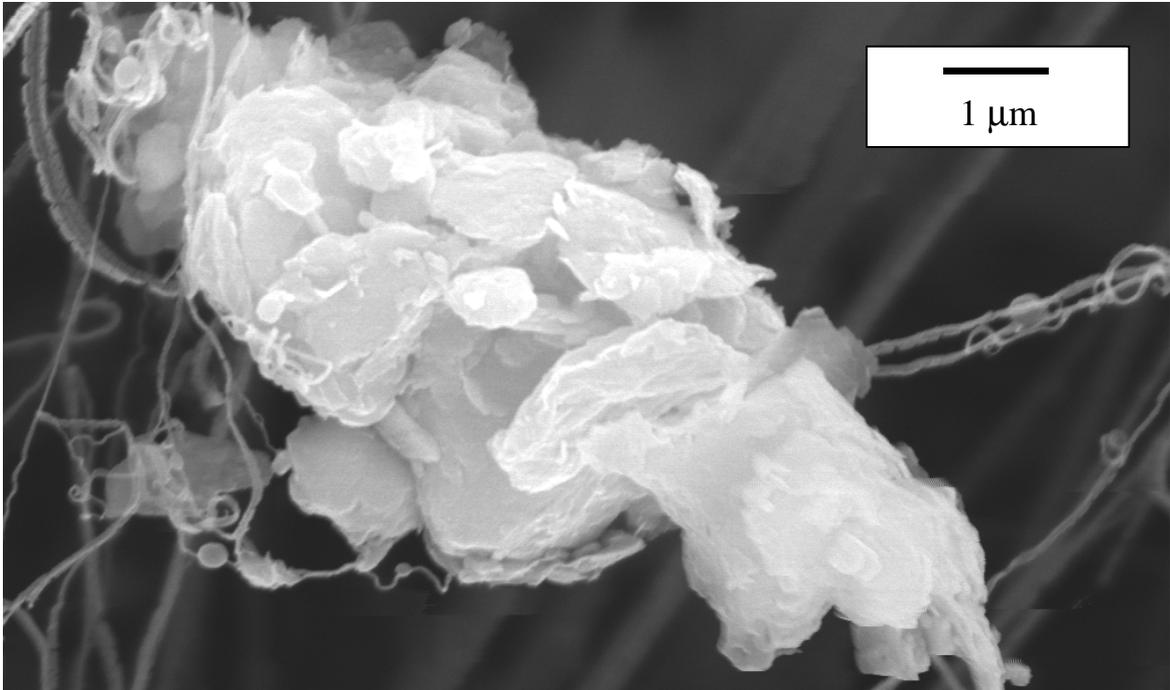
Figure A3. Spring sample – PM<sub>10</sub> - Collected at the High Level Forest Products Ltd. (HLFP) Site, Primary elements - Si, Al, Ca, Fe
