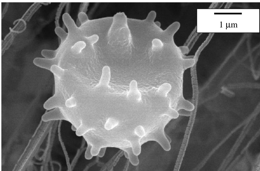
Figure A10. Example of an organic particle – PM<sub>10</sub> - collected at the Water Treatment Plant
