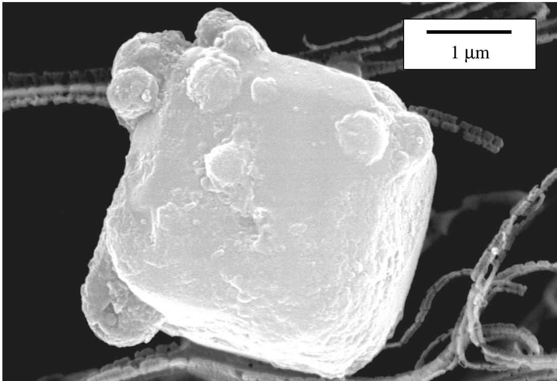
Figure A4. Spring sample – PM<sub>10</sub> - Collected at the hospital site, Primary elements - Si, Al, Ca, Na
