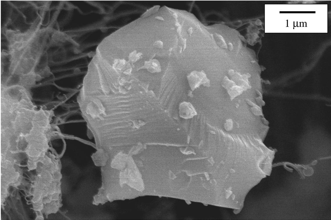
Figure A7. Fall Sample – PM<sub>10</sub> - Collected at the High Level Forest Products Ltd. (HLFP) site, Primary elements - Si, and trace Ca, Al, Ti
