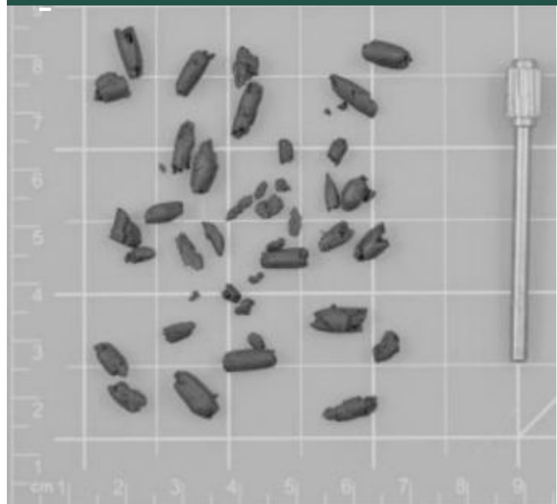
Figure 3: Sample snakes at plastic limit [5]
