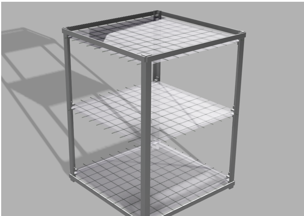
Figure 4.3: A 3D CAD model of a module containing 3 horizontal plastic scintillating panels, wavelength shifting fibres and a support structure. These modules would be combined to form the panel subregions shown in Figure 4.2.
