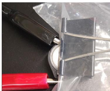
Figure S3.4. Coin cell setup for EIS measurement.
