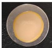
Figure S3.6. PVA6M after EIS measurements at 65 °C.
