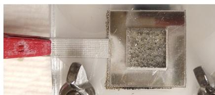
Figure S4.4. OER electrode using MBAA 0.3 after cycling test showing permeation of GPE through the Ni electrode.
