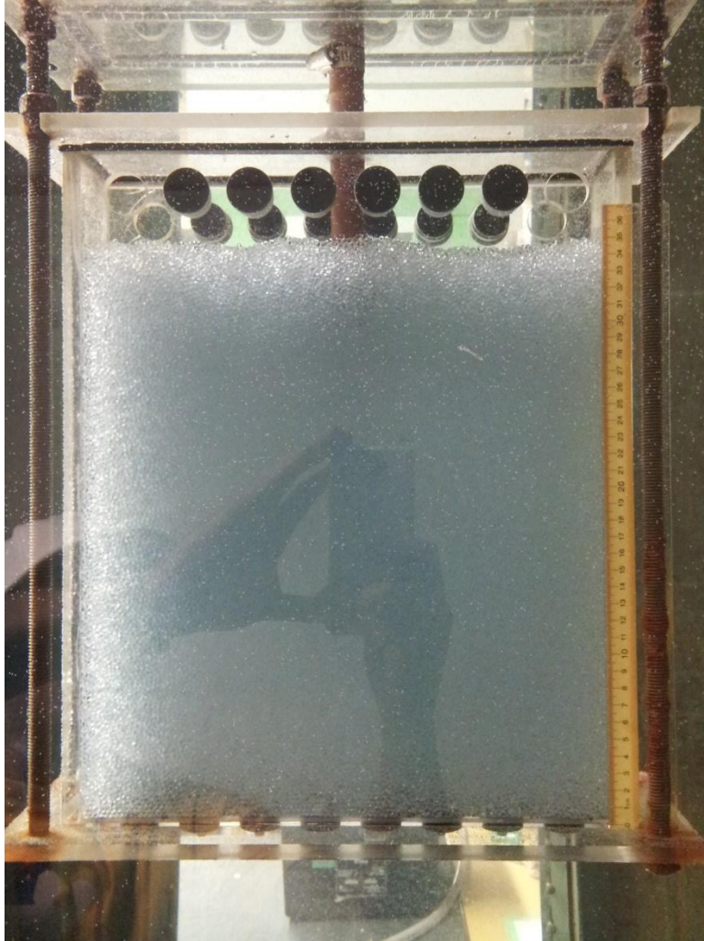
Figure 3-5: [color] A closeup of the research box submerged in the steel reservoir, supported by galvanized steel guide rods.
