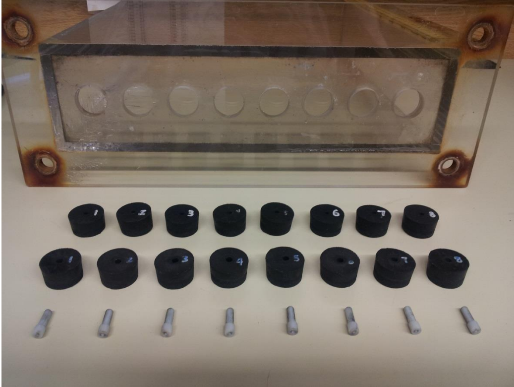
Figure 3-6: [color] Two rows of rubber one-hole stoppers used. The first row the stoppers have a hole diameter of 0.32 cm. The second row the stoppers have a hole diameter of 0.48 cm. The third row shows the ABS cylindrical inserts used to further reduce the hole diameter to 0.14 cm.
