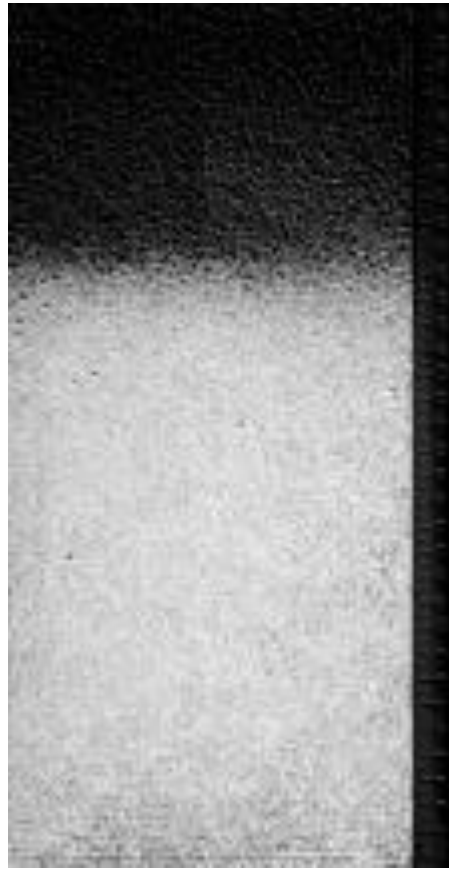
Figure 4-4: The result of an experimental image matrix being subtracted from a reference image matrix, known as a subtracted image.
