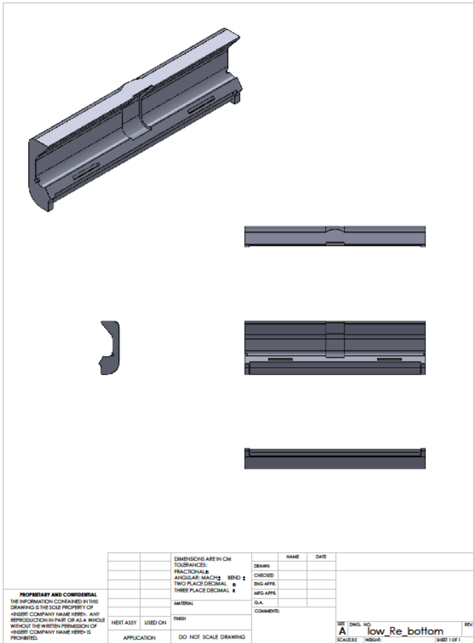
Figure C-15: Front, top, bottom, side and isometric view of the main bottom component of the order-1-Re line source.
