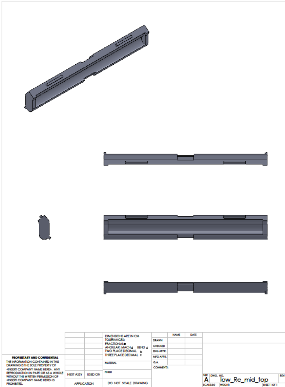
Figure C-16: Front, top, bottom, side and isometric view of secondary top component which is connected to the main top component shown in figure C-14.
