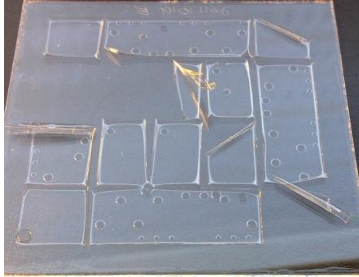
Figure C.2: Delamination post develop of 60°C PEB KMPR on silanized glass (4" borofloat glass substrate). From this result is it clear that a higher temperature PEB must be used during fabrication.
