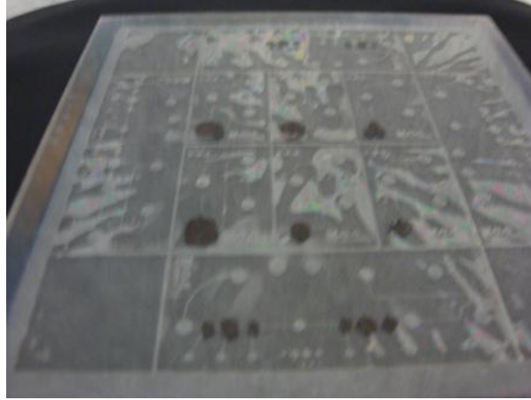
Figure C.11: Second bond of the full PC5k structure. Bond was performed at 90^{\circ}\text{C} for 15 minutes with a force of 5750N. In this case the bonding quality was poor due to the 120^{\circ}\text{C} bake performed after the first bonding step.
