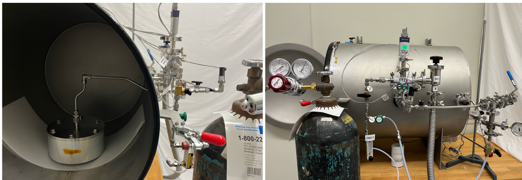
Figure 5.5: Experimental setup used to measure the permeation rates of lower mass noble gases and radon. The setup includes a vacuum holding tank, a permeation chamber, pressure transducers, and temperature sensors. A radon detector (not pictured) is used for the radon permeation rate measurement.
