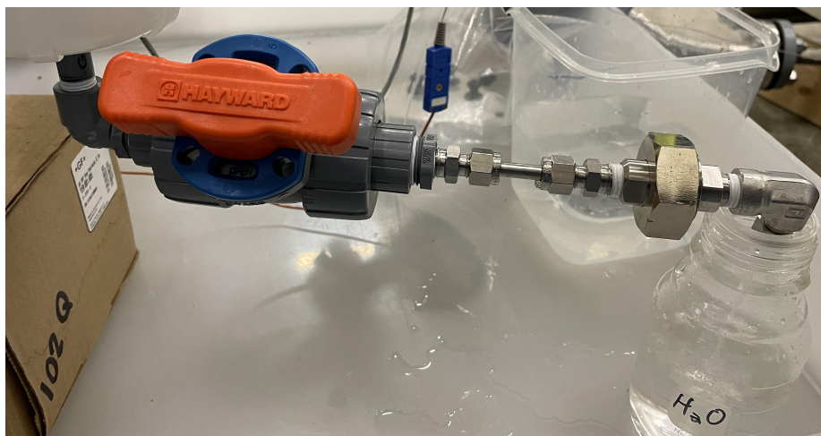
Figure 6.15: Sampling the UPW after a cleaning cycle of the outer quartz vessel.
