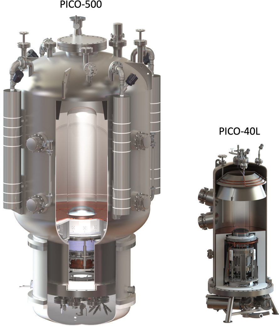
Figure 3.5: Cross-sectional CAD illustration of PICO-500, the next-generation bubble chamber detector compared to PICO-40L.
