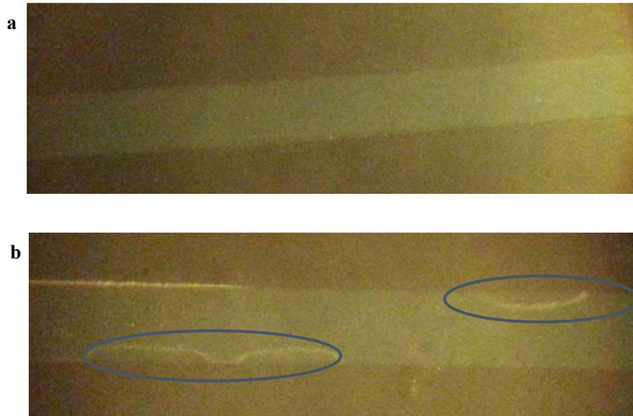
**Figure 2-12:** Image of 150 nm particle bed separation channels at **(a)** 30 V/cm (no crack was observed during separation), and **(b)** 65 V/cm (particles started to move from the walls of the chip, indicated by blue oval shaped). Both images were taken from the same chip during operation
