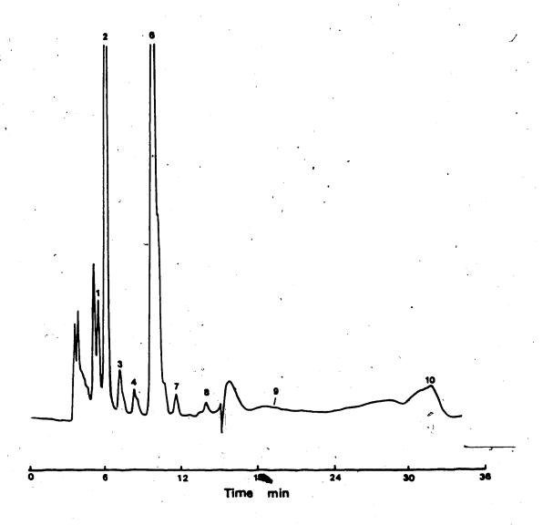
Figure 7.8. Liquid chromatogram of organic acids present in buttermilk powder.
