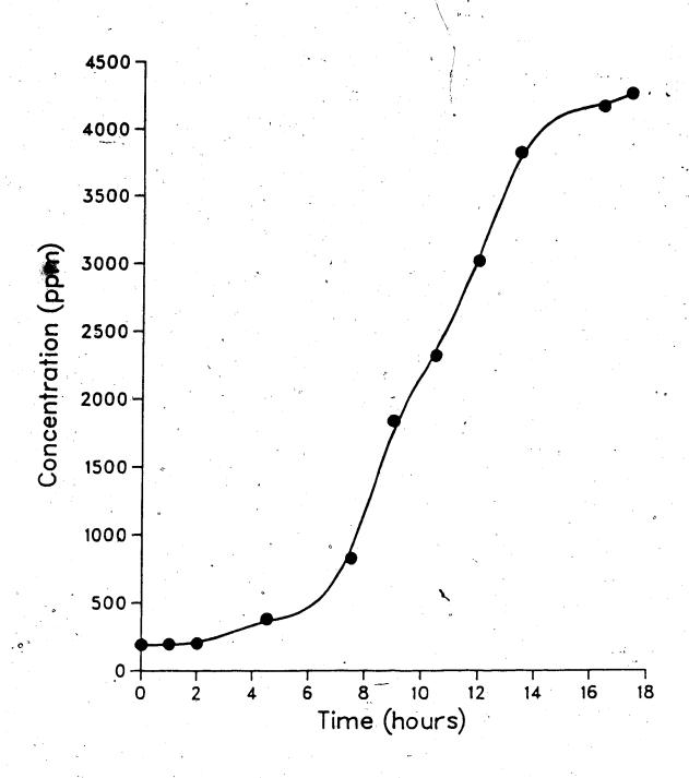
Figure 4.1 Lactic acid formation (ppm) during incubation of milk in the production of cultured buttermilk.
