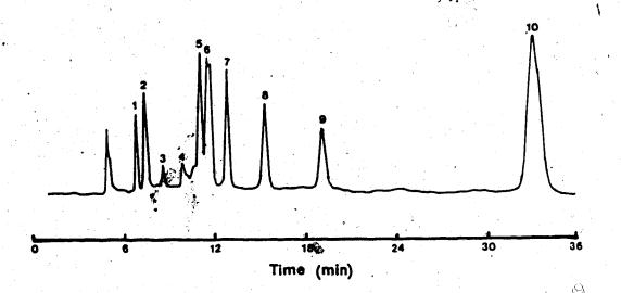
Figure 7.1. Liquid chromatogram of standard organic acids.
