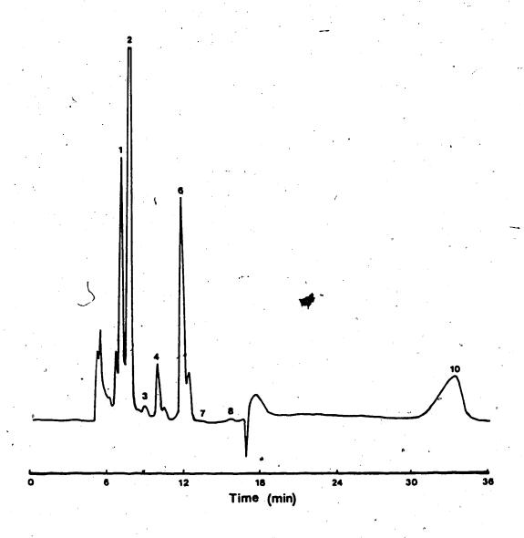
Figure 7.4. Liquid chromatogram of organic acids present in partly skimmed milk (2% BF).
