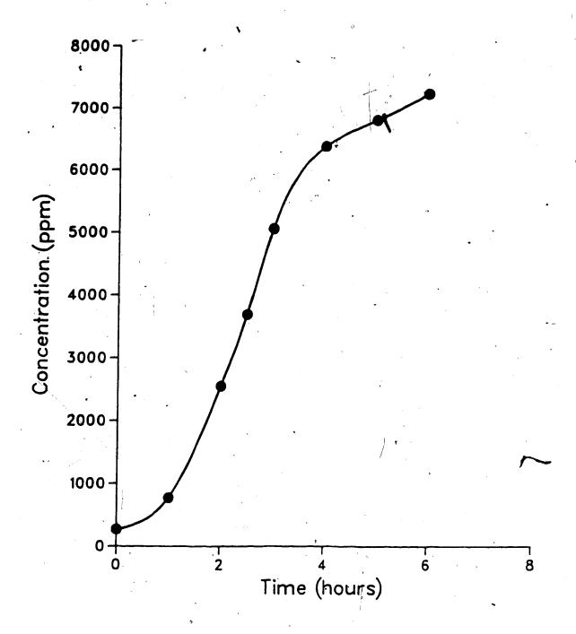
Figure 4.3 Lactic acid formation (ppm) during incubation of milk in the production of yogurt.
