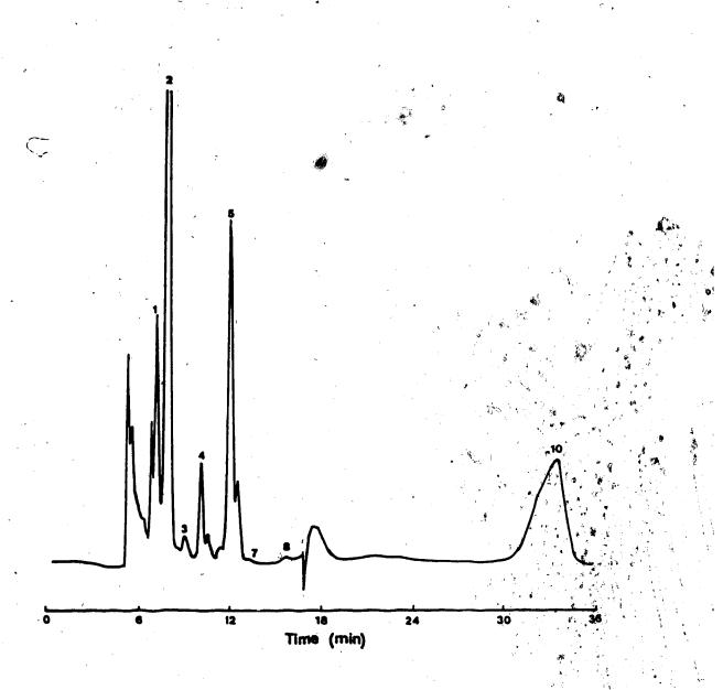
Figure 7.9. Liquid chromatogram of organic acids present in skim milk powder.
