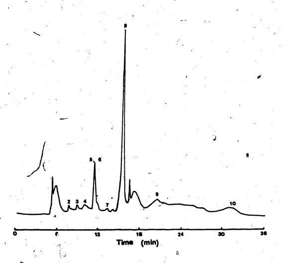
Figure 7.30. Liquid chromatogram of organic acids present in French Roquefort.
