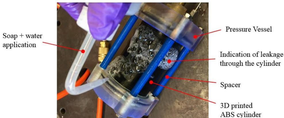
Figure 9: A digital image showing a mix of water and soap to check if leakage was present during the experiment through the body of the cylinder.
