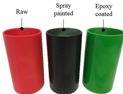
Figure 18: The three different cylinder samples with a wall thickness of 1/8” used on the pressure measurement.
