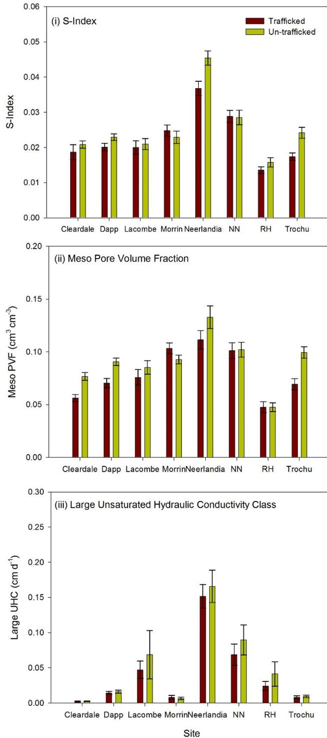
**Fig. 1.4** The soil physical quality as described by (i) S-Index (ii) Meso pore volume fraction (PVF) and (ii) Large unsaturated hydraulic conductivity (UHC) class in trafficked (IT) and un-trafficked (CTF) treatments for each site (NN: New Norway; RH: Rolling Hills). The soil physical quality metric S-Index is well correlated with the soil characteristics of meso PVF and large UHC. The mean values of each soil parameter is shown with their respective standard error values.
