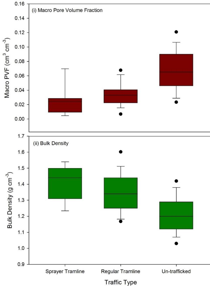
**Fig 3.2** Comparison of (i) macro pore volume fraction (PVF) and (ii) bulk density across traffic types (sprayer tramline, CTF tramline and un-trafficked zones) that are commonly displayed in a CTF landscape.
