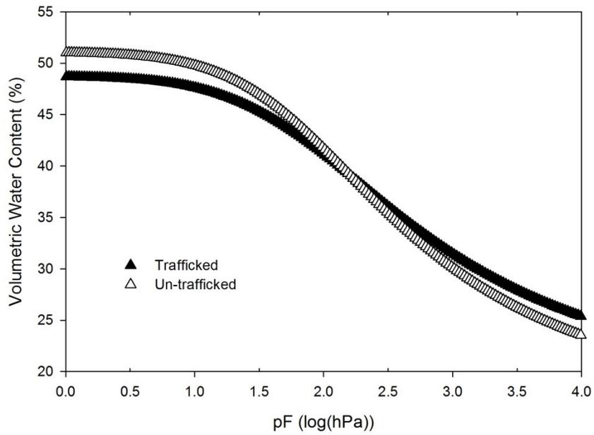
**Fig. 1.3** Water retention curve of the sites compared between trafficked (IT) and un-trafficked (CTF) treatments. The curves display van Genuchten modeled values based upon the data range of the measured values (n= 200).
