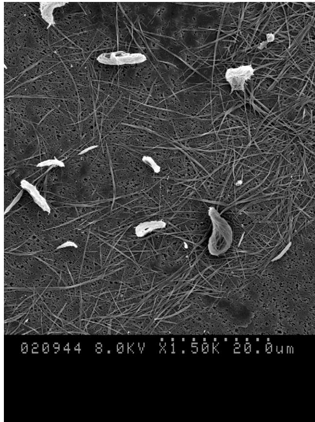
Figure 33: SEM image of particles generated with dry air at 14.7 l/min at 1500x magnification
