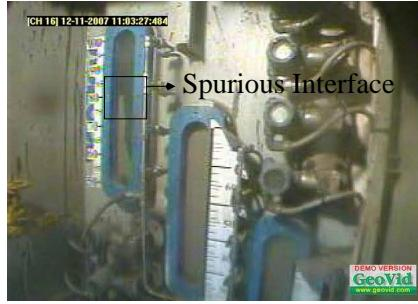
Figure 4.3: Process abnormality in the separation cell
