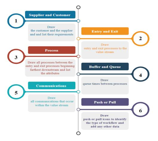
Figure 7. Development of current state map for VSM adjusted from Tapping and Shuker (2003)
