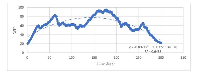
Figure 38. WIP in the design process.
