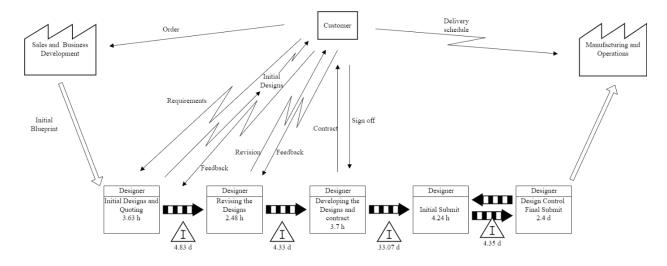
Figure 36. The process duration for the value stream current state map
