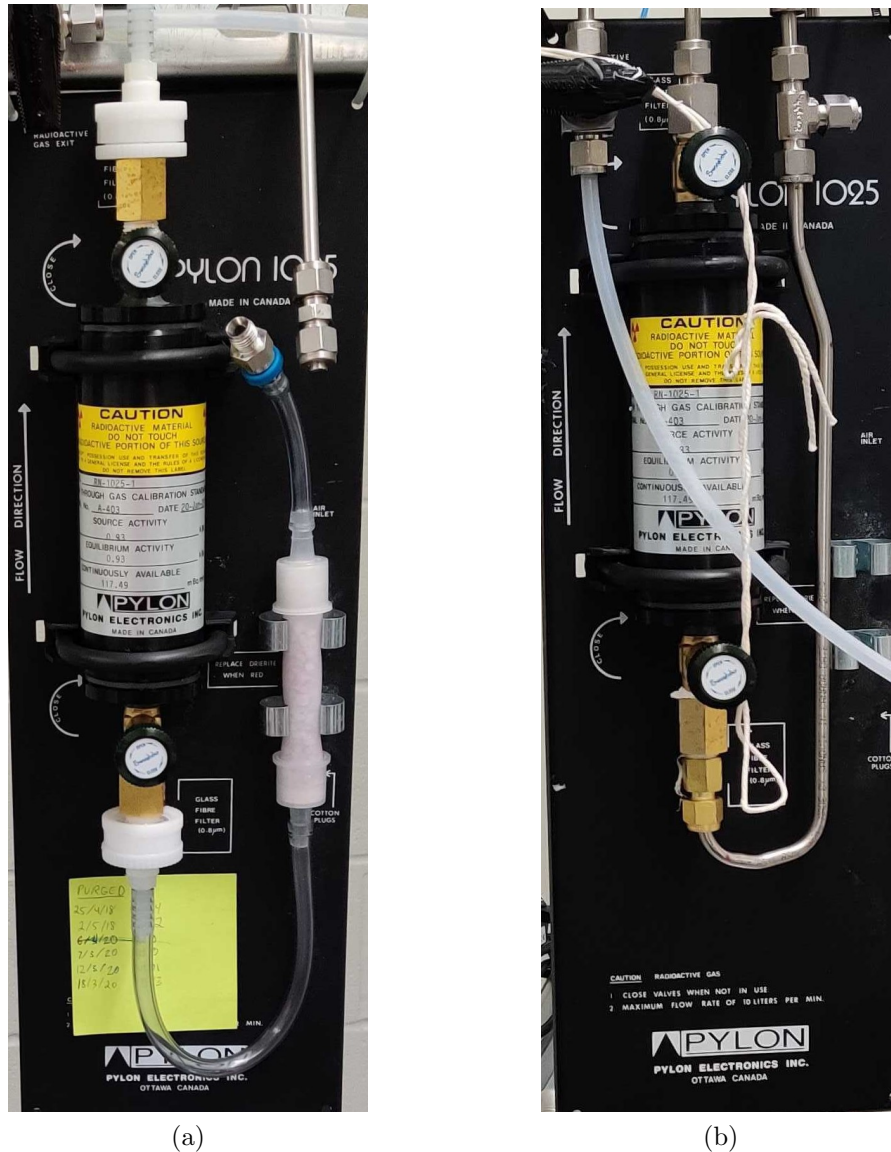
Figure 5.10: The radon source: (a) as produced by Pylon. (b) modified with stainless steel piping. The desiccant (right side white tube in (a)) was replaced with an inline desiccant that uses Swagelok connections in a different section of the RTS.
