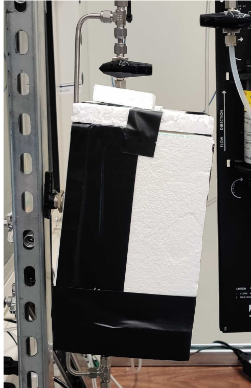
Figure 6.10: The cooling system for the radon trap is a customized polystyrene box capable of holding 4.5 kg of dry ice pellets.
