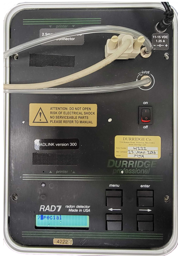
Figure 5.7: An image of the RAD7 external interface. Vinyl tubing is attached to the inlet and outlet and the serial port interfaces with the CAPTURE ® (DURRIDGE Company Inc) software. The RAD7 can be controlled via the LCD screen and buttons.
