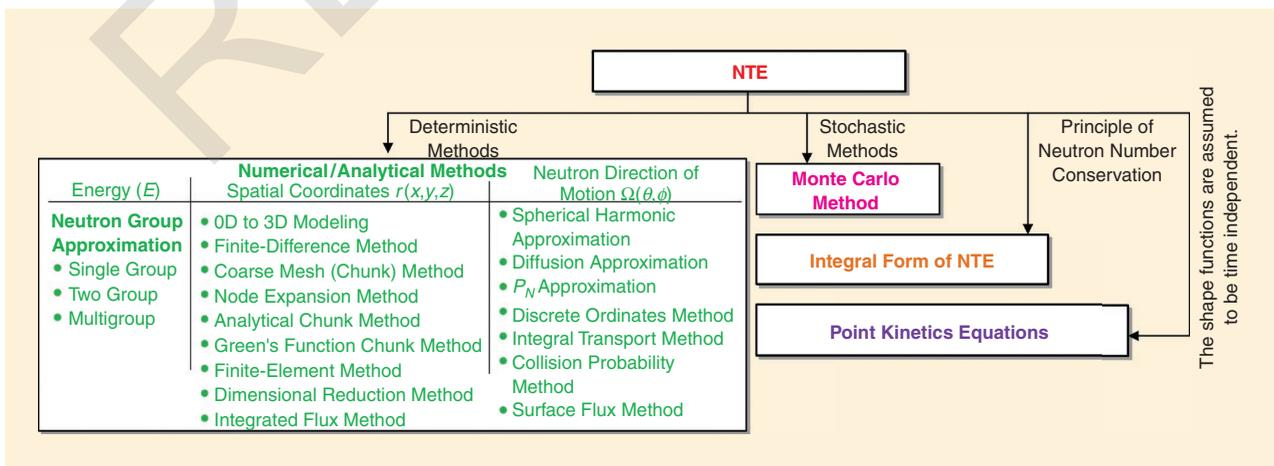
Figure 6. Core modeling and numerical calculation methods.
