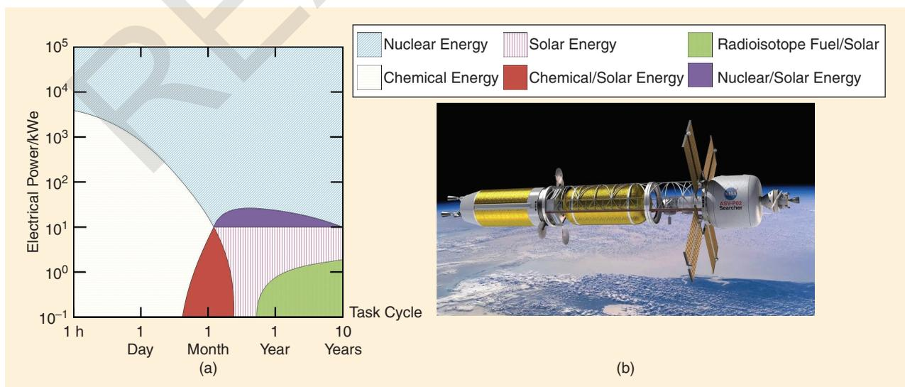
Figure 3. (a) The applicability of space energy sources and mission cycles. (b) A nuclear thermal propulsion spacecraft. (Image source: NASA.)
