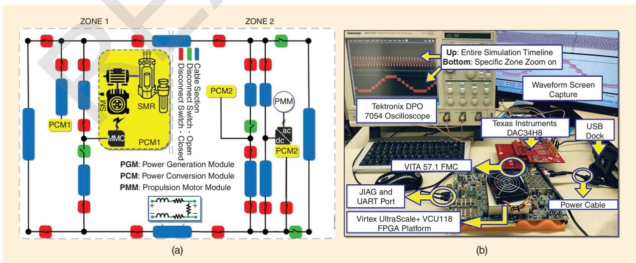
**Figure 9.** (a) A modified conceptual two-zone MVdc SPS equipped with an SMR. (b) An SMR RTDT on an FPGA prototyping platform. JTAG: Joint Test Action Group; UART: universal asynchronous receiver-transmitter.
