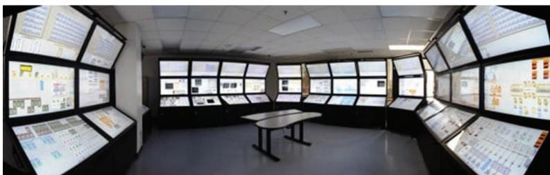
Figure 8. The full-scale layout of the Human Systems Simulation Laboratory glass-top simulator. (Source: Idaho National Laboratory.)
