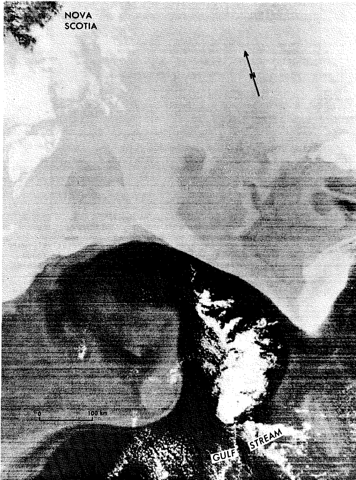
PHOTOGRAPH 5. VHRR thermal-infrared image showing temperature variations in the Gulf Stream. The gray-scale range is -10^{\circ}\text{C} (white) to +20^{\circ}\text{C} (black). Original scale 1:4,500,000. (Photo courtesy of AES Satellite Data Laboratory)
