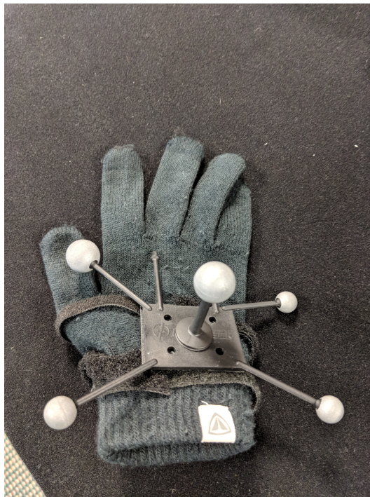
Figure 3.7: The first version of our hand tracking made using Optitrack tracking system
