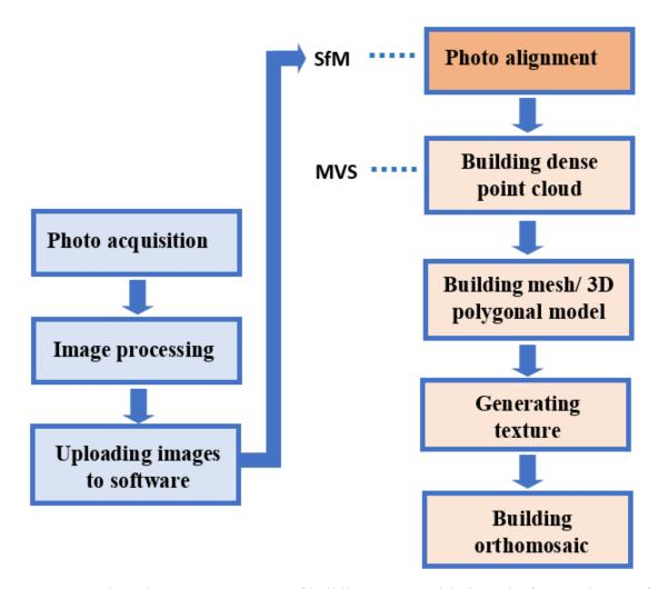
**Figure 2.4.** Flow chart presents stages of building a 3D model via Agisoft Metashape Software. SfM and MVS algorithm-based stages are indicated (modified from Hayes et al., 2017).
