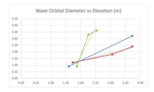
**Figure 3.8.** Graph showing wave orbital diameter values (x-axis) plotted against elevation (y-axis) values. Measurement elevations increase corresponds to shallowing in depth. The shallower depths represent higher wave orbital diameter values. Red line: East Ridge measurements, Blue line: West Ridge measurements, Green line: South Ridge measurements.
