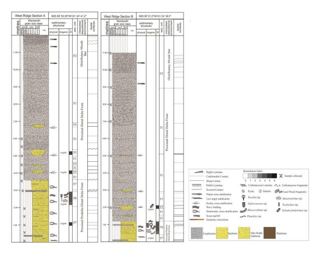
**Figure 2.9.** Lithologic strip logs representing facies thicknesses measured on West Ridge. From section A (basinward) to section B (landward) decrease in the abundance of sandy facies is observable.
