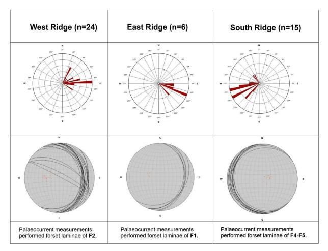
**Figure 2.8.** Rose and equal area stereonet plots representing palaeoflow directions for West, East and South ridges respectively. West and East Ridge measurements indicate eastwards dominant palaeoflow on the other hand South Ridge measurements indicate westwards dominant palaeoflow.
