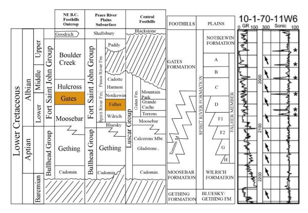
**Figure 2.1.** Lower Cretaceous Albian stratigraphic chart (Smith et al., 1984). 10-1-70-11W6 gamma-ray log on the right shows coarsening upward parasequences separated by coal spikes from Falher A through H (after Smith et al., 1984; Zonneveld and Moslow, 2004).
