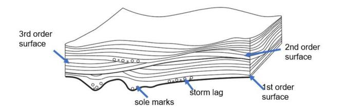
Figure 3.3. HCS illustration showing order of surfaces (modified from Harms et al., 1975).
