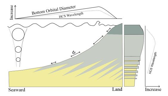
**Figure 3.7.** Diagram shows wave orbital diameter vs. HCS wavelength change (Yang and Dalrymple et al., 2006).
