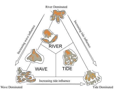
**Figure 2.20.** Tripartite model showing delta geometries changing related to relative energies of shallow marine processes (Galloway, 1975).
