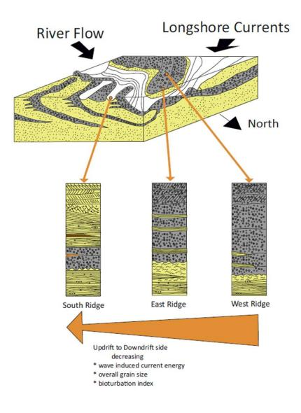
**Figure 2.22.** Model shows deflection of river mouth from symmetric to asymmetric due to longshore transport. Vertical sections representing hypothetical palaeo-depositional locations of West, East, and South ridges (modified from Bhattacharya et al., 2003) Downdrift deflection of river mouth is caused by longshore currents. Gray facies represent conglomerate and yellow represents sandstone.
