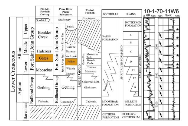
**Figure 1.1.** Lower Cretaceous Albian stratigraphic chart (Smith et al., 1984). 10-1-70-11W6 gamma-ray log on the right shows coarsening upward parasequences separated by coal spikes from Falher A through H (after Smith et al., 1984; Zonneveld and Moslow, 2004).
