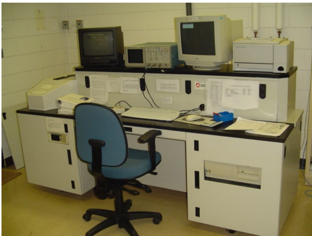
Figure 2-4: AB Sciex Voyager Elite MALDI-Time of Flight (TOF) mass spectrometer. Picture is downloaded from http://www.chem.ualberta.ca/~masspec/instr.htm .
