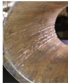
Longitudinal banding in bends and straight section - *EC feature*
