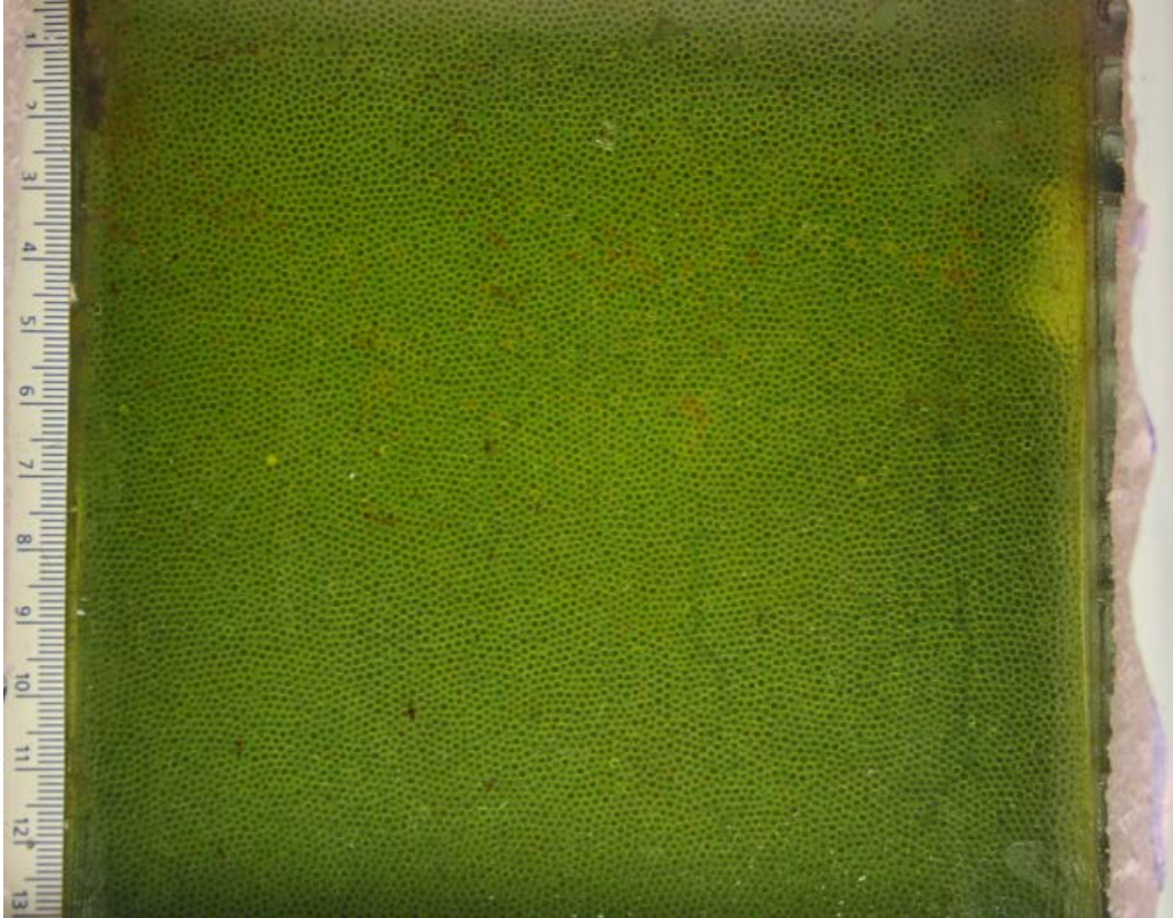
Figure G.1 Sample image of the saturated freezing cell filed with admixture of water and BAND-ADE Sawing fluid at 12% volume ratio with water. Fluorescein was added for coloring.
