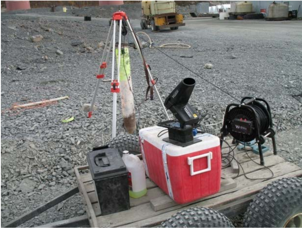
Figure E.4 Well-vu camera setup in MW 6 at the tank farm area.
