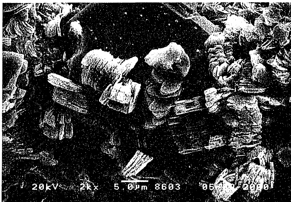
Figure 2.4. (a) Sketch of the lattice structure of kaolinite (Grim, 1953). (b) Electron micrograph of kaolinite material (Mineralogy Database. http://webmineral.com/data/Kaolinite.shtml . Accessed August 2005)
