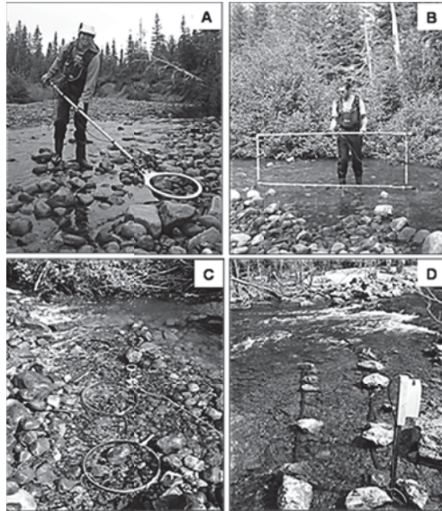
Fig. 7. Different types of PIT systems: A) portable system, B) large portable system, C) flat-bed antenna grid (during installation) and D) single-point stationary system. Photo credits: Patricia Johnston (A, B, C) and Jean-Nicolas Bujold (D). Modified from Johnston & Bergeron (2009).
