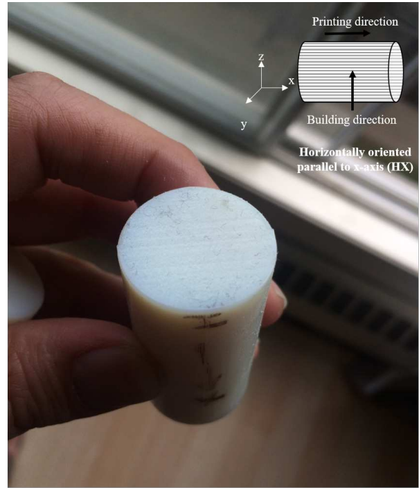
Figure A.8: 3D-Printed layers orientation (different finish depending on the building orientation).
