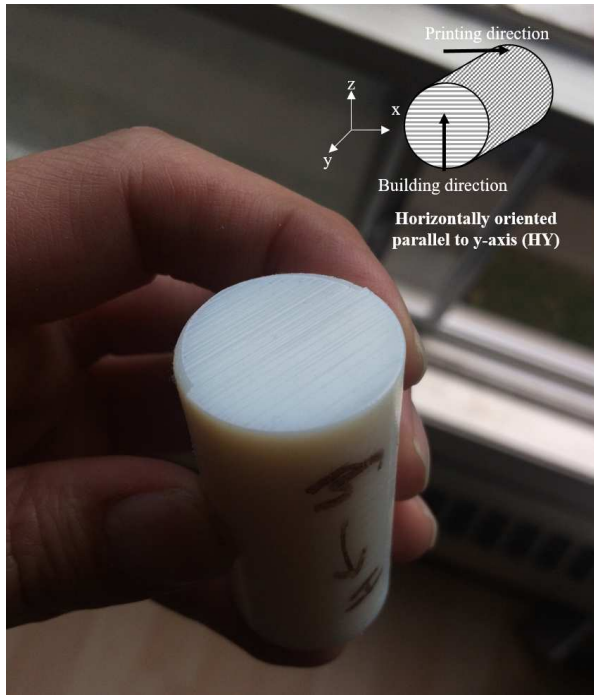
Figure A.8: 3D-Printed layers orientation (different finish depending on the building orientation).
