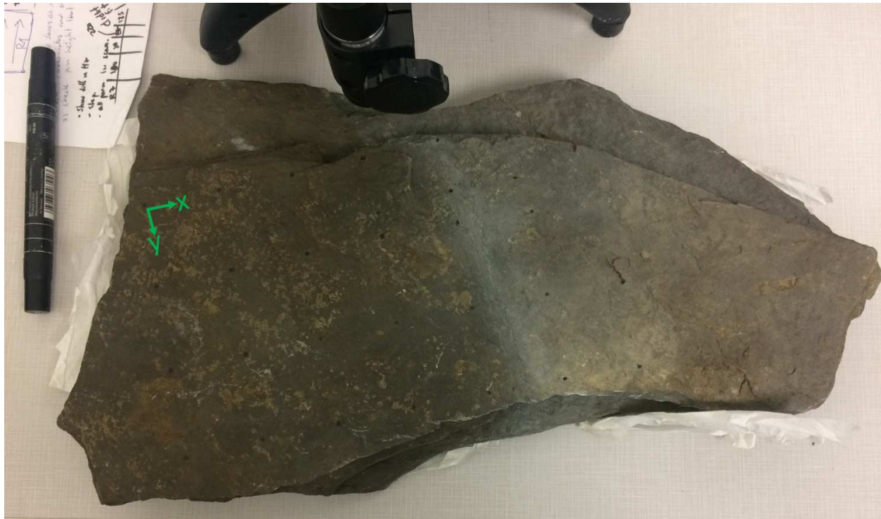
Figure D.1: Sample preparation prior to surface measurements with a profilometer.
