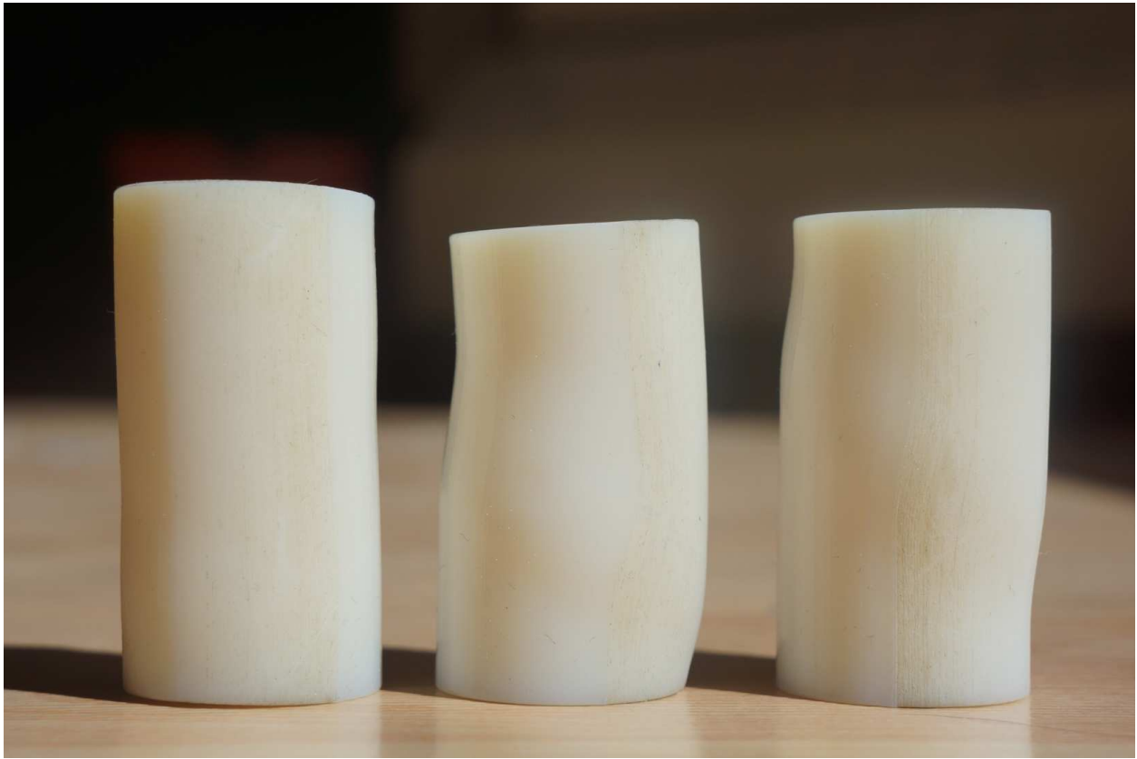
Figure A.7: VeroWhite samples oriented parallel to x-axis (HX) after UCS tests.
