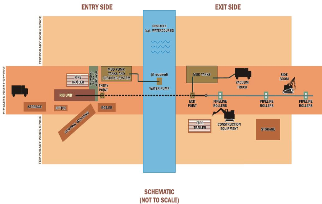
Figure 13: Schematic of Horizontal Directional Drilling (Canadian Association of Petroleum Producers, 2004)
