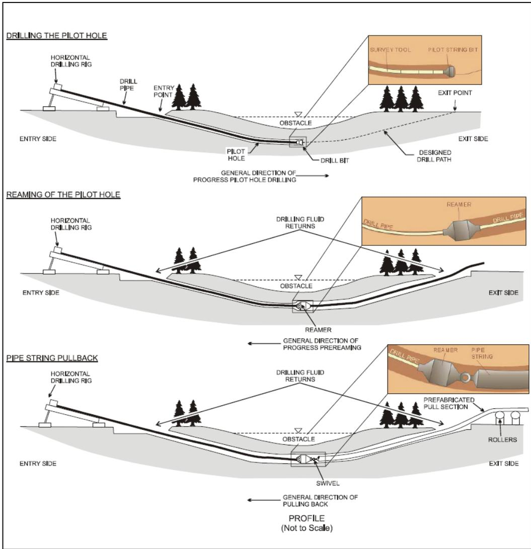
Figure 14: Schematic of Horizontal Directional Drilling (Canadian Association of Petroleum Producers, 2004)
