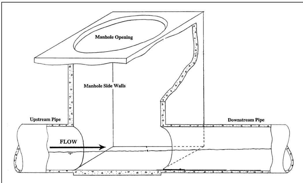
Figure 15: Illustration of Manhole at Stormwater Pipe Connection (Adapted from Maheepala, et al. 1998)
