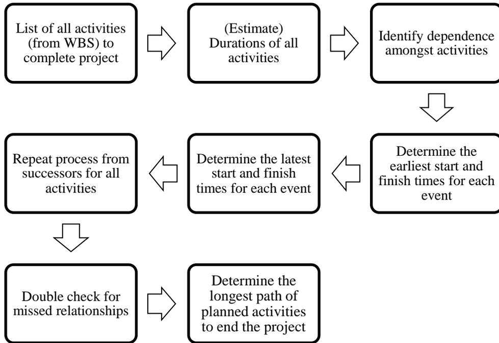
Figure 7: CPM Methodology (Adapted from Prensa, 2002)
