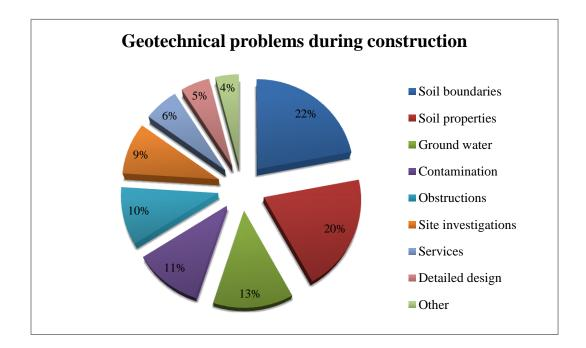
Figure 11: Geotechnical Risks during Construction (Adapted from Clayton, 2001)
