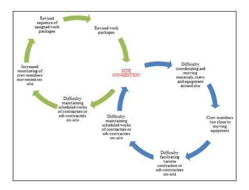
Figure 9: Causal Loop Showing Overcrowding Risks (Adapted from Spillane, 2011)
