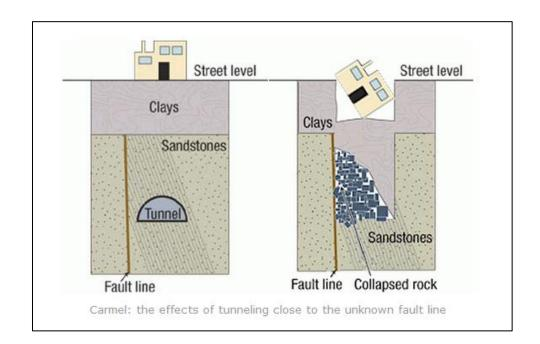
Figure 12: Illustration of the Tunnel Collapse in Barcelona, Spain, (Barcelona Field Studies Centre, 2005)
