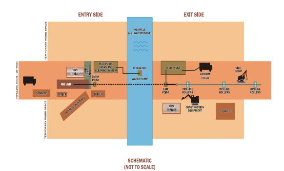
Figure 13: Schematic of Horizontal Directional Drilling (Canadian Association of Petroleum Producers, 2004)
