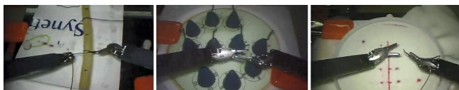
Fig. 4. Sample frames of video data in the JIGSAWS dataset for three elementary tasks (From left to right): knot-tying task, needle-passing task, and suturing task.
