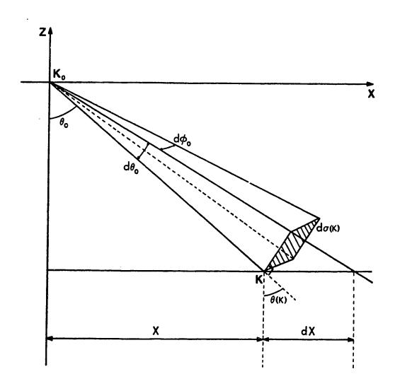
Figure 4: Ray tube between  $K_0$  and K for a homogeneous medium
