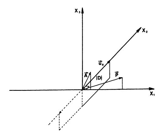
Figure 2: Parameters for SH waves particle motion
