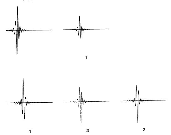
S1S1 VP1=1.850 VP2=2.190 VS1=0.300 VS2=0.900 DEN1=1.920 DEN2=2.300 ANGLE OF INCIDENCE= 23.0
