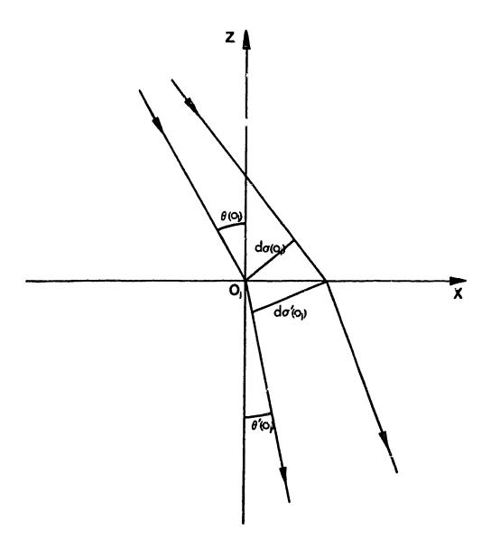
Figure 6: Change in the cross-sectional area of the ray tube at an interface
