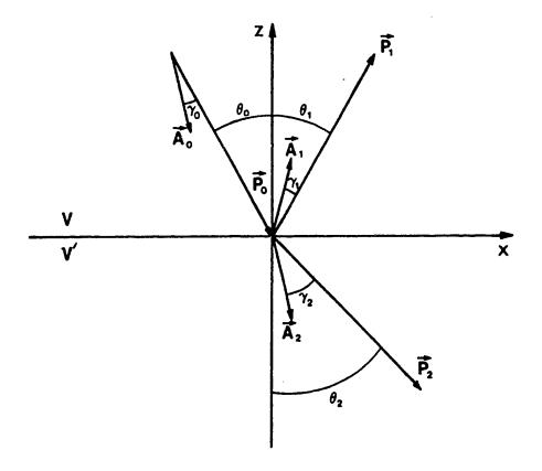
Figure 1: Incident, reflected and transmitted rays at a boundary separating two anelastic media
