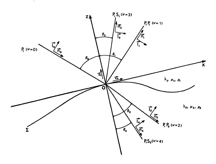
Figure 7: Intersection of the plane of incidence  $\qquad \qquad \text{of the ray with the boundary } \Sigma$
