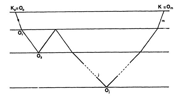
Figure 5: A typical ray in homogeneous layered medium
