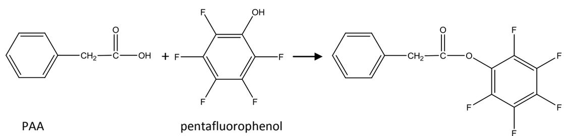
Figure 4. Derivatization of PAA with pentafluorophenol produces a fluorinated ester.
