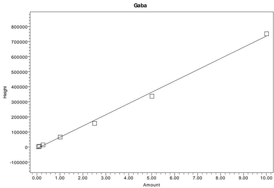
Figure 17. Typical standard curve for GABA.
