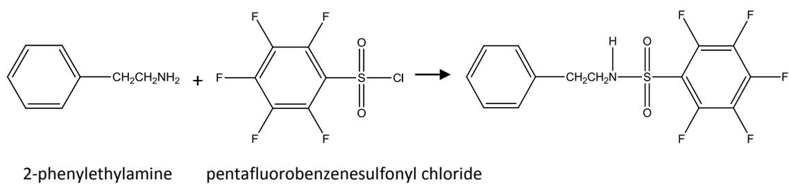
Figure 3. Derivatization of PEA with pentafluorobenzenesulfonyl chloride
