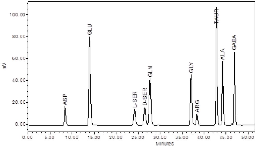
Figure 13. Example of an HPLC amino acid trace from the assay used for analysis of amino acid levels. ASP = L-aspartate; GLU =L-glutamate; L-SER = L-serine; D-SER = D-serine; GLN = L-glutamine; GLY = glycine; ARG = L-arginine; TAUR = L-taurine; ALA =L-alanine; GABA =  $\gamma$ -aminobutyric acid. Hereafter in the thesis, D- and L- are only used with D- and L-serine.
