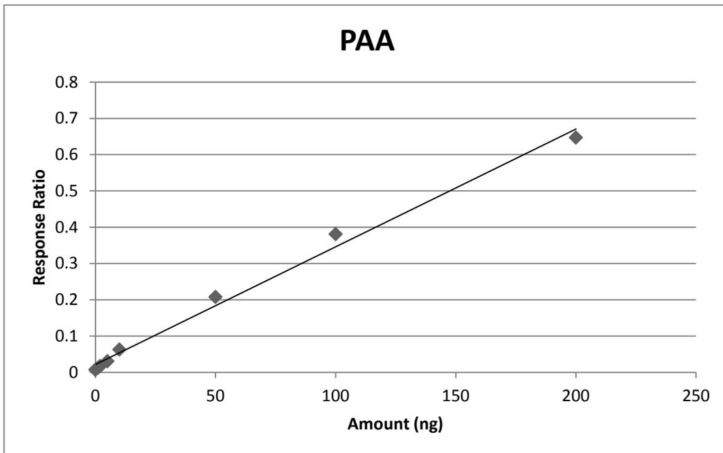
Figure 9. Typical standard curve for the PAA assay.
