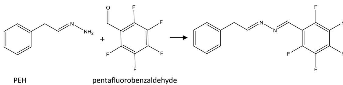
Figure 2. Derivatization of PEH with pentafluorobenzaldehyde.
