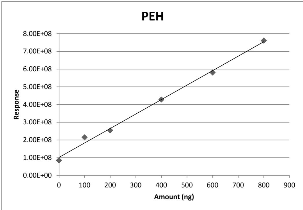
Figure 6. Typical standard curve for the PEH assay.
