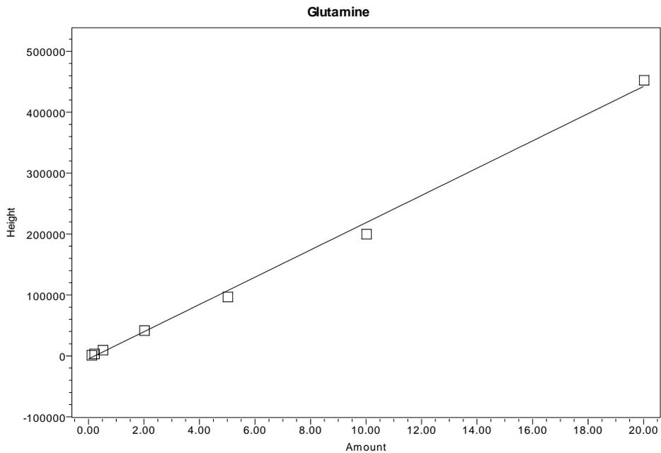
Figure 19. Typical standard curve for glutamine.
