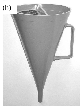
Figure 3.4: Preparation of slurry (a); Marsh Flow Cone (b)
