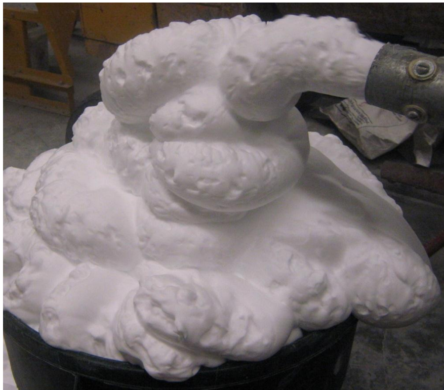
Figure 3.3: Stable foams coming out through the nozzle
