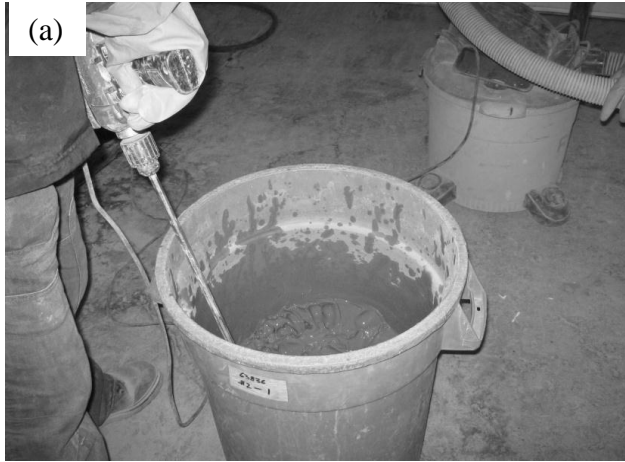
Figure 3.4: Preparation of slurry (a); Marsh Flow Cone (b)
