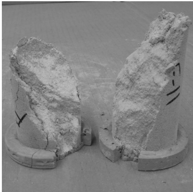
Figure 4.3: Compression test on plain cement-based foam cylinders (cast density 750 \text{ kg/m}^3 )
