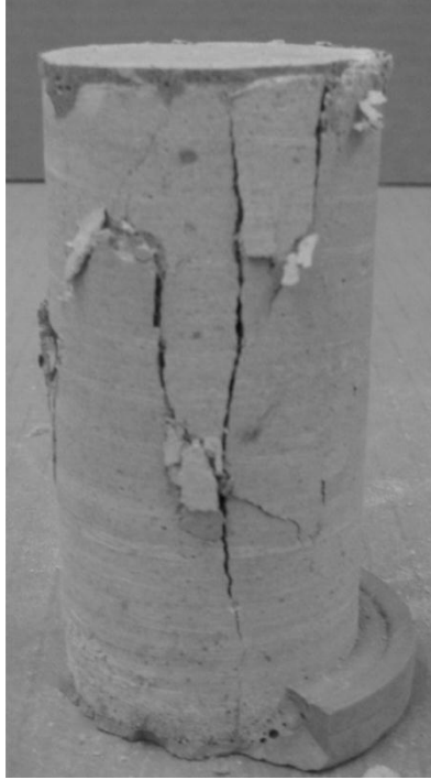
Figure 4.4: Compression test on fibre-reinforced cement-based foam cylinders (cast density 1200 \text{ kg/m}^3 )
