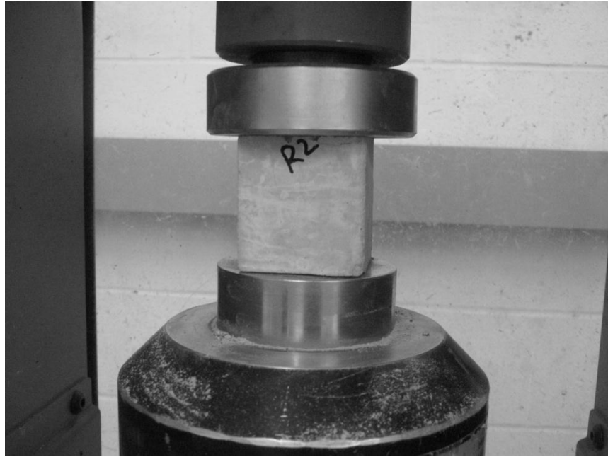
Figure 3.14: Compression test on cube specimens
