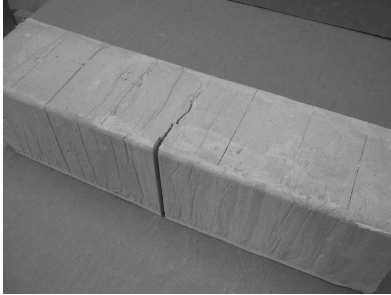
Figure 4.12: Quasi-static flexure test on fibre-reinforced cement-based foam (cast density 750 \text{ kg/m}^3 )
