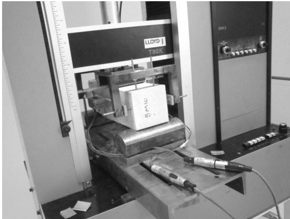
Figure 3.8: Screw-type test machine used for compression and quasi-static flexure test
