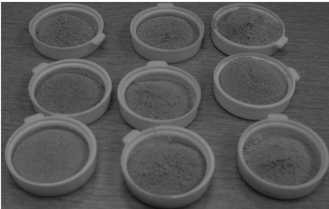
Figure 3.17: Powdered specimens used in X-Ray Diffraction
