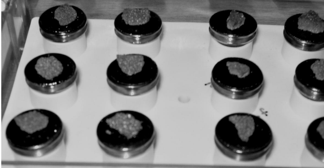
Figure 3.16: Specimens coated with gold for Scanning Electron Microscopy
