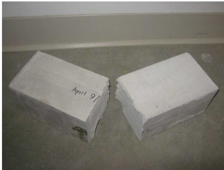
Figure 4.9: Quasi-static flexure test on plain cement-based foam (cast density 750 \text{ kg/m}^3 )
