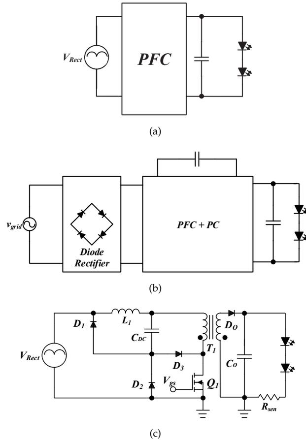
FIGURE 2.10: Single stage PFC topologies;
