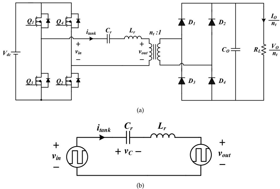
FIGURE 4.11: Series resonant converter: (a) Circuit Schematic, (b) simplified circuit
