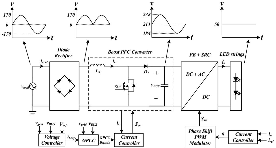
FIGURE 3.9: PFC + SRC control block diagram and Voltage levels
