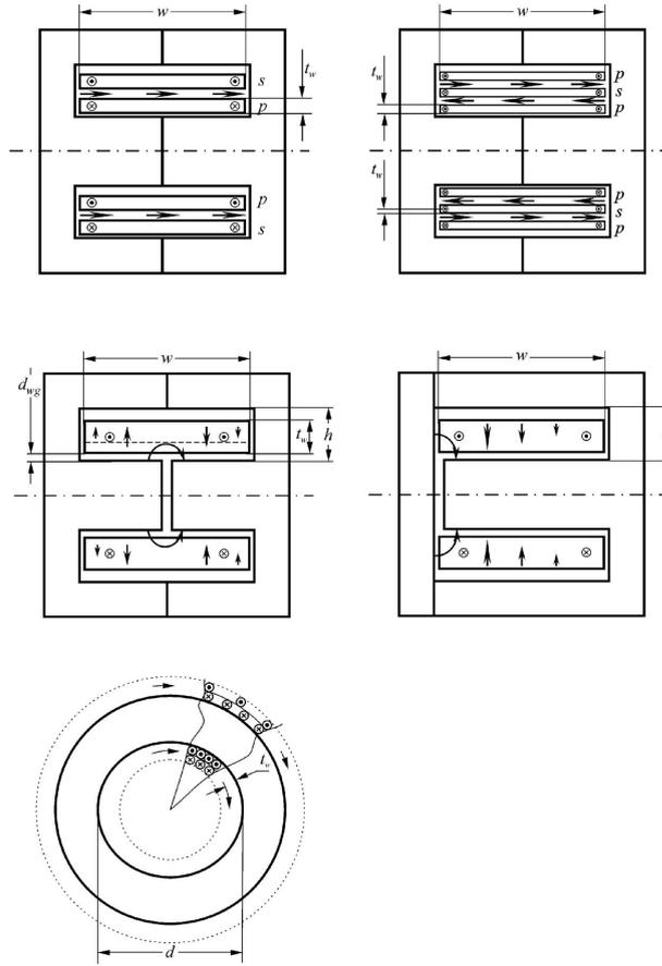
FIGURE 5.13: Magnetic Component Shape and field directions [4]
