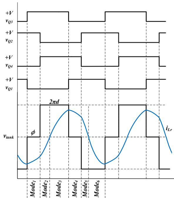
FIGURE 4.2: Phase shift Switching Pattern, resonant Tank Input Voltage, Current, and SRC Modes of Operation
