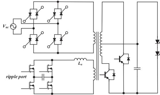
FIGURE 3.6: Isolated energy storage concept
