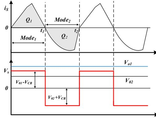
FIGURE A.11: Current and voltages on the secondary side of transformer
