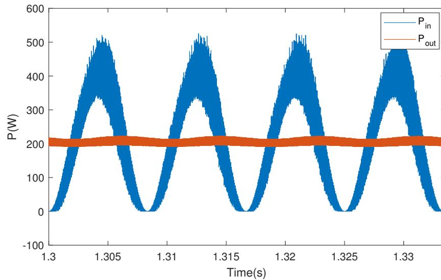
FIGURE 3.11: Power decoupling in LED driver : Input alternating power vs output power of 4 LED channels
