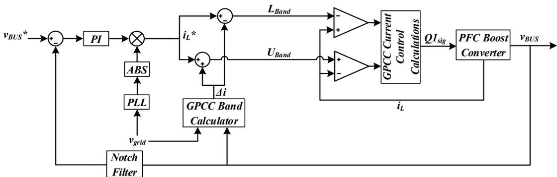
FIGURE 2.12: PFC control diagram
