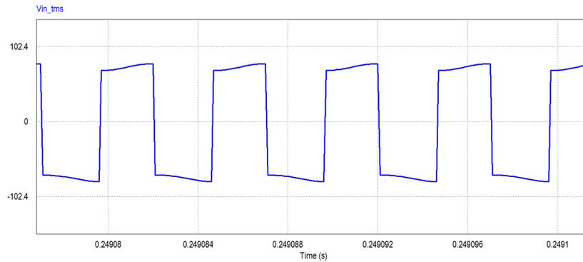
FIGURE 5.4: Primary winding voltage of resonant transformer
