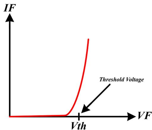
FIGURE A.1: V-I characteristic curve of LED
