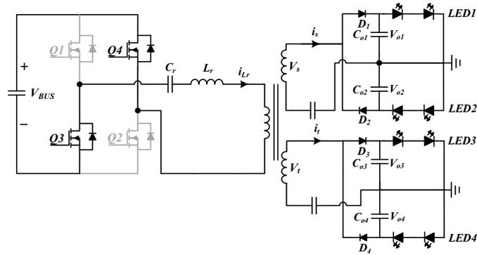
FIGURE 4.10: Mode 5 and 6 of resonant converter operation
