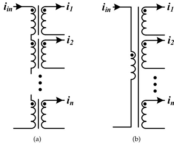
FIGURE A.7: Current sharing approaches with transformer: (a) Series connected transformers and (b) Multiple output transformer
