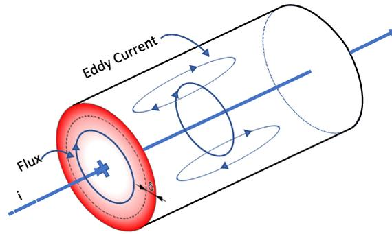
FIGURE 5.8: Eddy current in conductors
