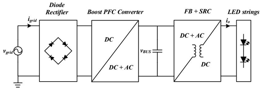
FIGURE 1.3: Power circuit block diagram of the proposed LED driver
