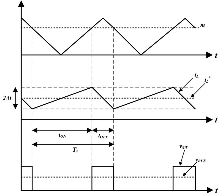
FIGURE 2.15: Step up PFC converter: carrier signal, inductor current and output voltage
