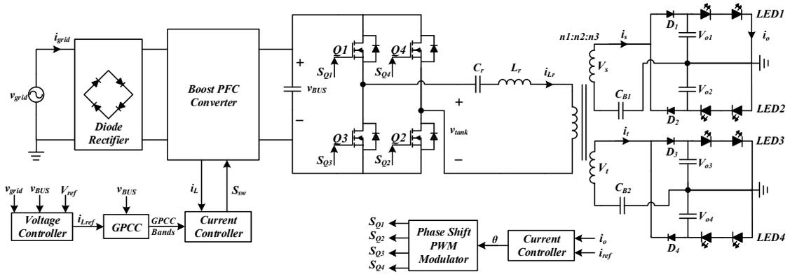
FIGURE 4.1: Series Resonant Converter topology
