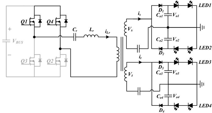
FIGURE 4.3: Mode 1 of resonant converter operation
