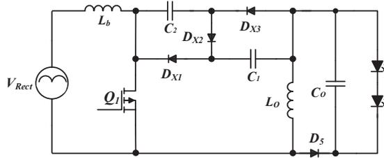
FIGURE 3.7: Sepic-derived PFC stage based on valley fill circuit.
