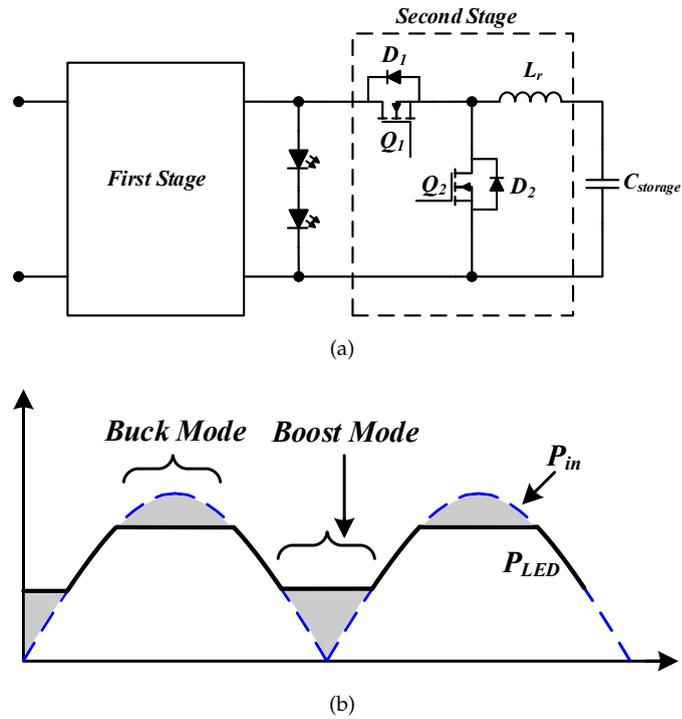
FIGURE 3.2: Reduced power processing approach with cascaded topology
