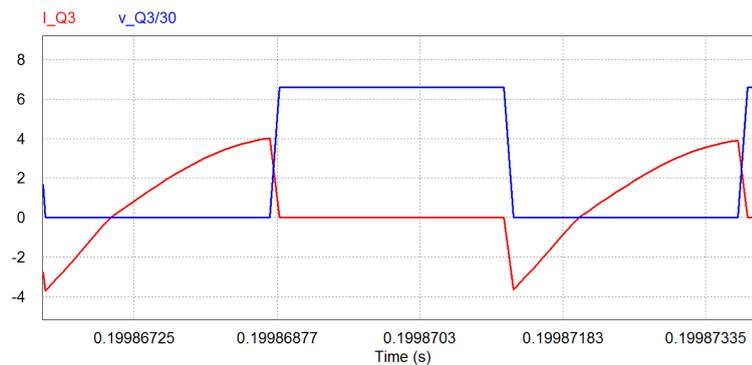
FIGURE 4.7: Zero voltage switching in switch  $Q_3$
