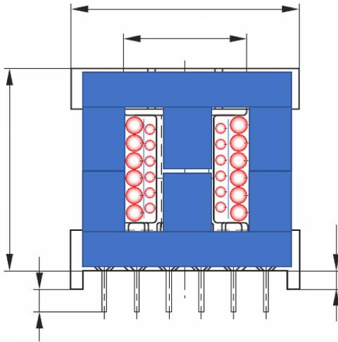
FIGURE 5.5: Bobbin, Core, and Wires Structure
