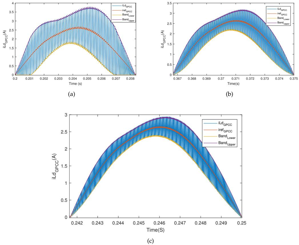
FIGURE 2.19: GPCC constructed Bands corresponding to (a)  $i_{Ld} = 1 \text{ mH}$ , (b)  $i_{Ld} = 2 \text{ mH}$ , (c)  $i_{Ld} = 3 \text{ mH}$
