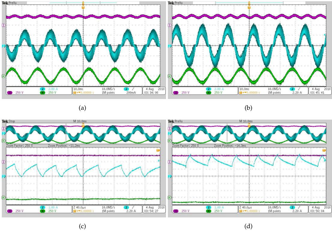
FIGURE 2.20: GPCC controlled Power Factor Correction Stage waveforms are output voltage, input current, and input voltage:
