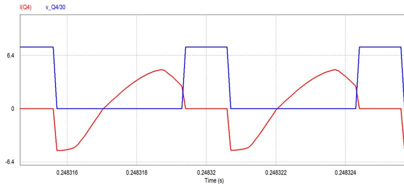
FIGURE 4.9: Zero voltage switching in switch  $Q_4$
