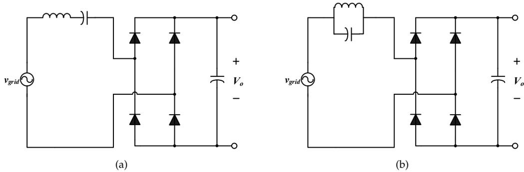
FIGURE 2.4: Rectifier with resonant structure PFC
