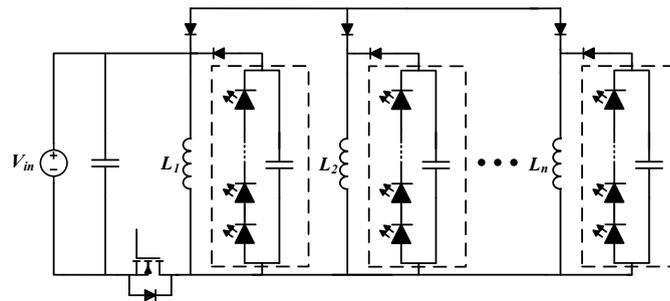
FIGURE A.6: Buck-Boost topology using inductor current sharing in [5]
