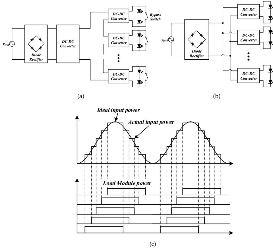
FIGURE 3.5: Load Modularization; (a) Series module connections, (b) Parallel module connection, (c) Input and load output power
