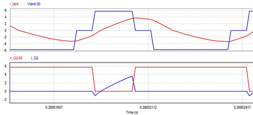
FIGURE 4.5: Zero voltage switching in switch  $Q_2$
