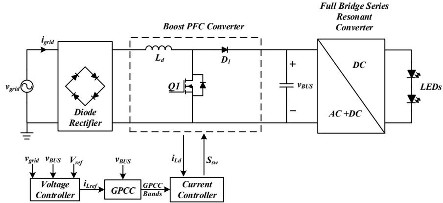
FIGURE 2.1: Boost power factor correction in Two stage LED drive
