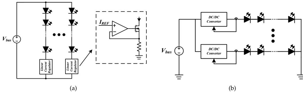
FIGURE A.2: Active current sharing approaches: (a) Linear and (b) Switch-mode
