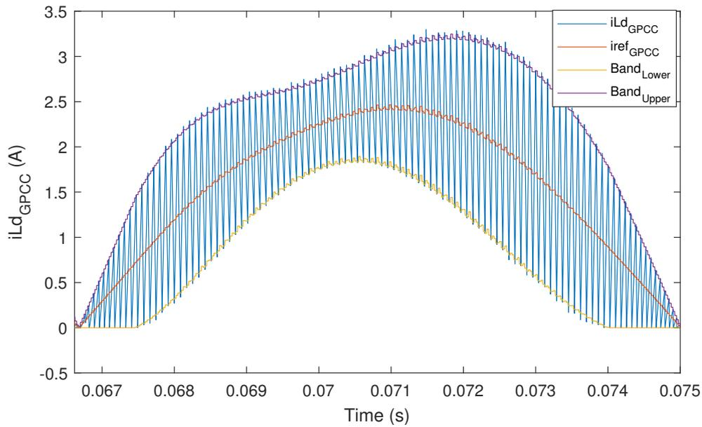
FIGURE 2.16: PFC inductor current based on GPCC control method
