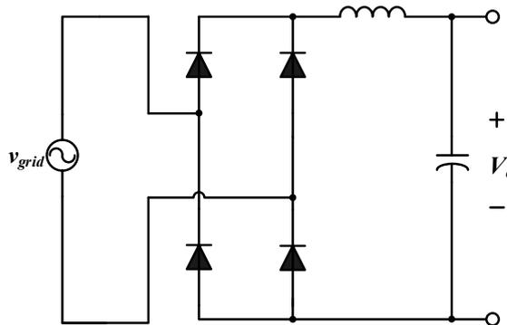
FIGURE 2.5: Rectifier with DC side inductor
