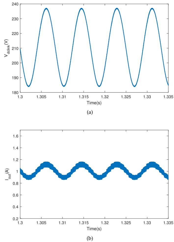
FIGURE 3.12: Power Decoupling in LED driver: (a) DC link voltage, (b) LED string current
