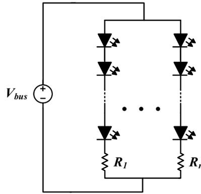
FIGURE A.3: current division method for resistive current sharing
