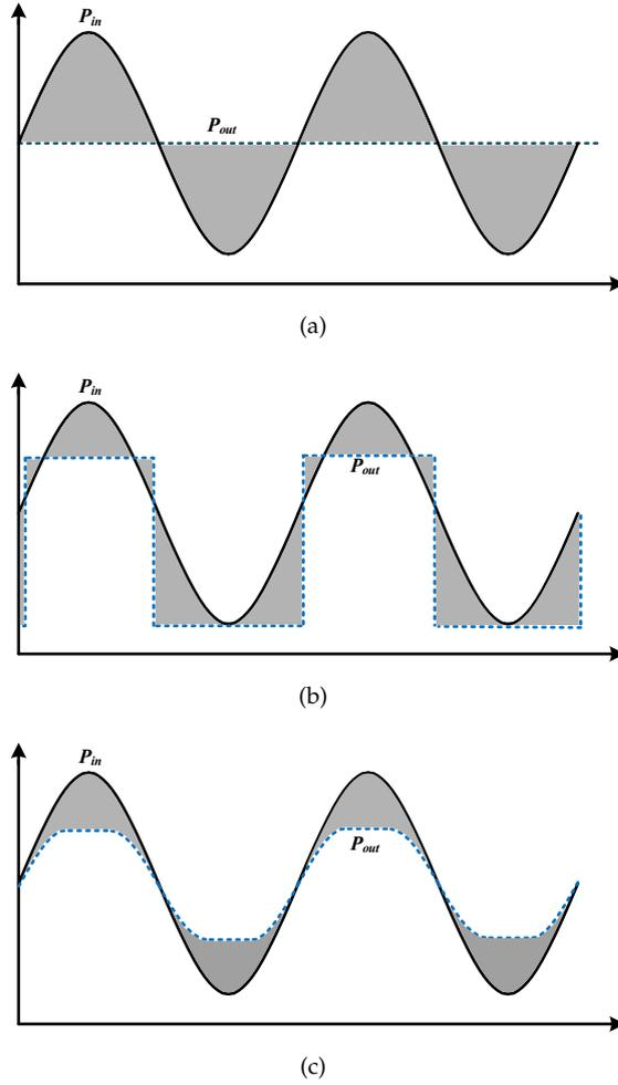
FIGURE 3.1: Output power utilizing different driving currents; (a) Sinusoidal waveform: input power vs output power with constant dc driving current, (b) output power with square wave driving current, (c) output power with dc biased harmonic combined driving current
