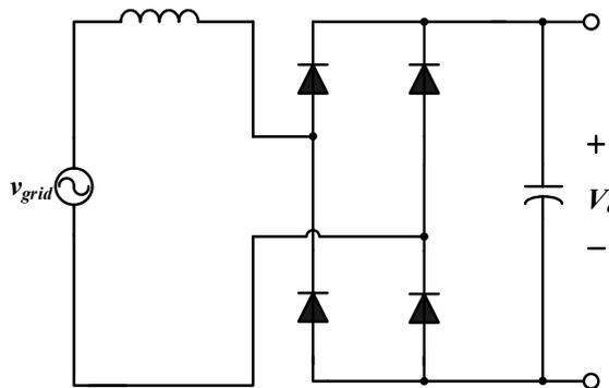
FIGURE 2.3: Rectifier with AC side inductor
