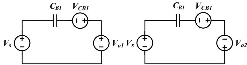
FIGURE A.12: Simplified circuit in Mode 1 and Mode 2 of current sharing
