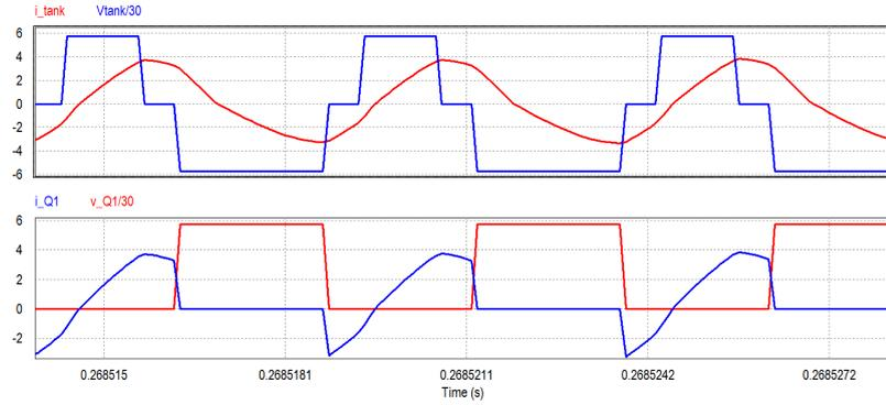
FIGURE 4.4: Zero voltage switching in switch  $Q_1$
