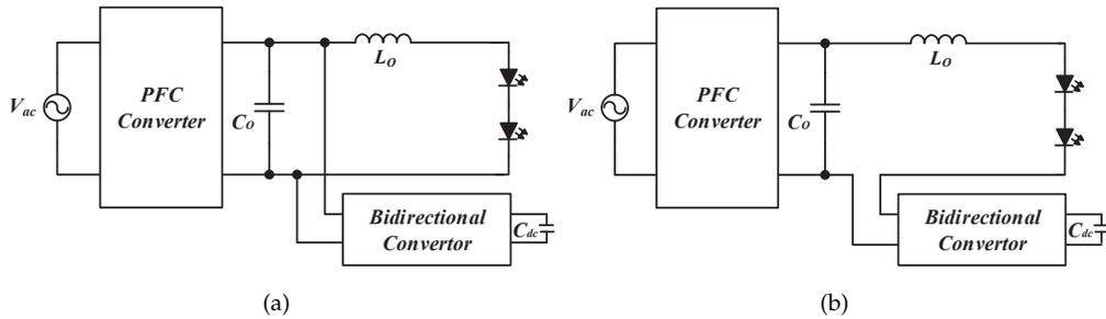
FIGURE 3.8: Electrolytic capacitor elimination using bidirectional converter in (a) parallel or (b) series connection with LEDs
