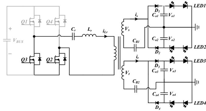
FIGURE 4.8: Mode 4 of resonant converter operation
