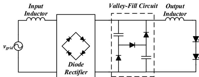
FIGURE 3.4: LED driver with inductive energy storage
