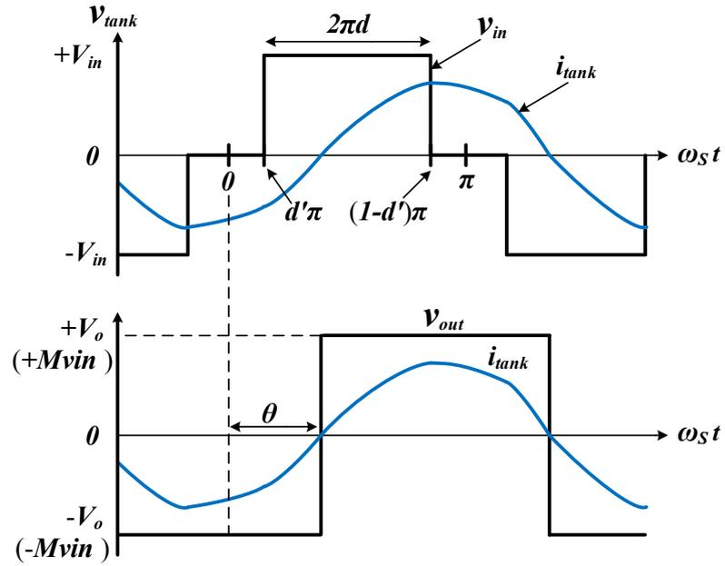
FIGURE 4.12: Typical waveforms of series resonant converter
