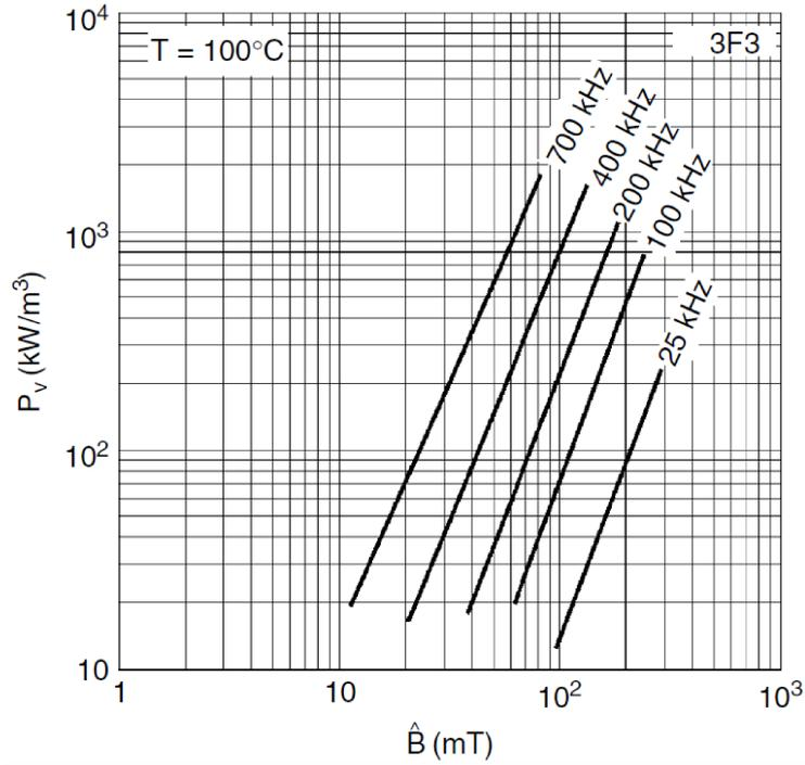
FIGURE 5.3: Core loss per volume as a function of Peak flux density for 3F3 ferrite material @100°C and operating frequency as the changing parameter [33]
