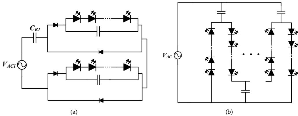
FIGURE A.5: Capacitor charge balancing method for current sharing: (a) two-string structure and (b) multiple-strings structure
