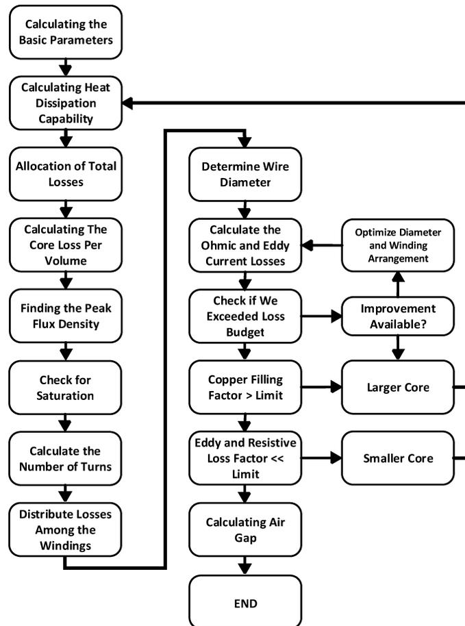
FIGURE 5.1: Magnetic Design Flow Chart for Non-Saturated Components
