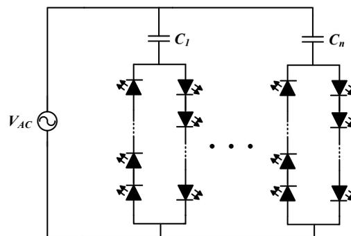
FIGURE A.4: current division method for capacitive current sharing
