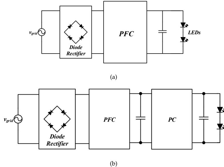
FIGURE 1.2: LED driver topologies;
