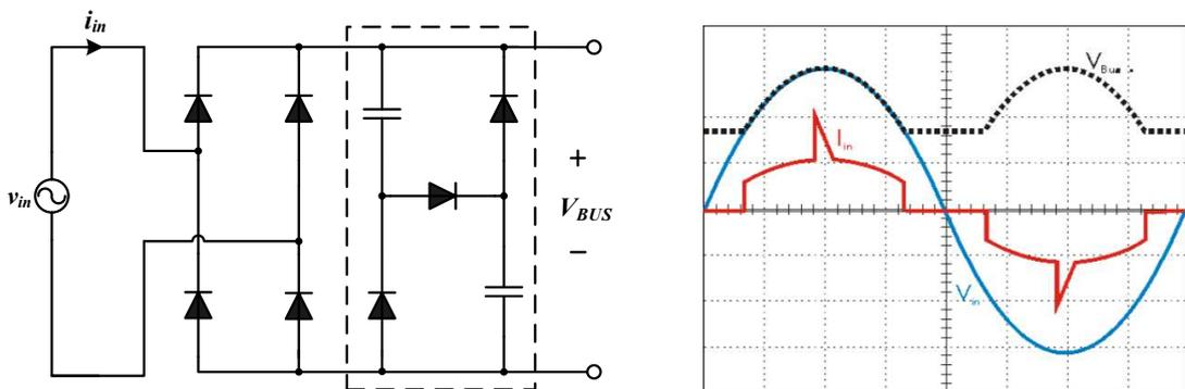
FIGURE 2.7: Valley-fill PFC topology and V-I waveforms[2]
