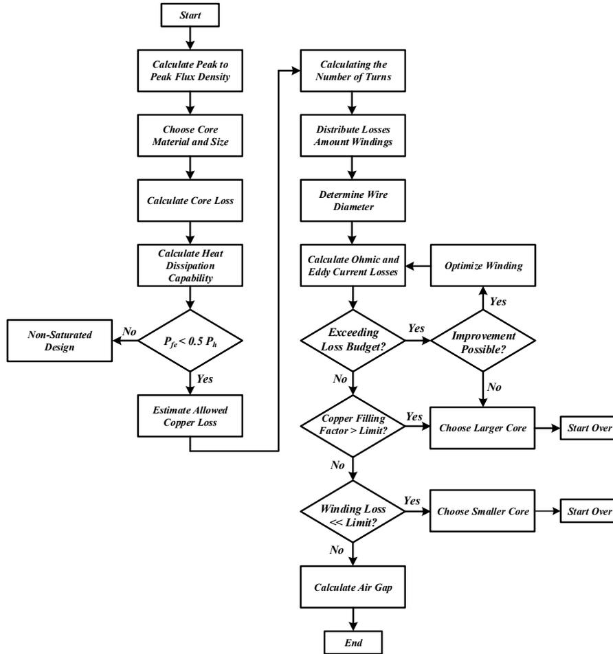
FIGURE 5.14: Flow chart for magnetic design with saturation limit
