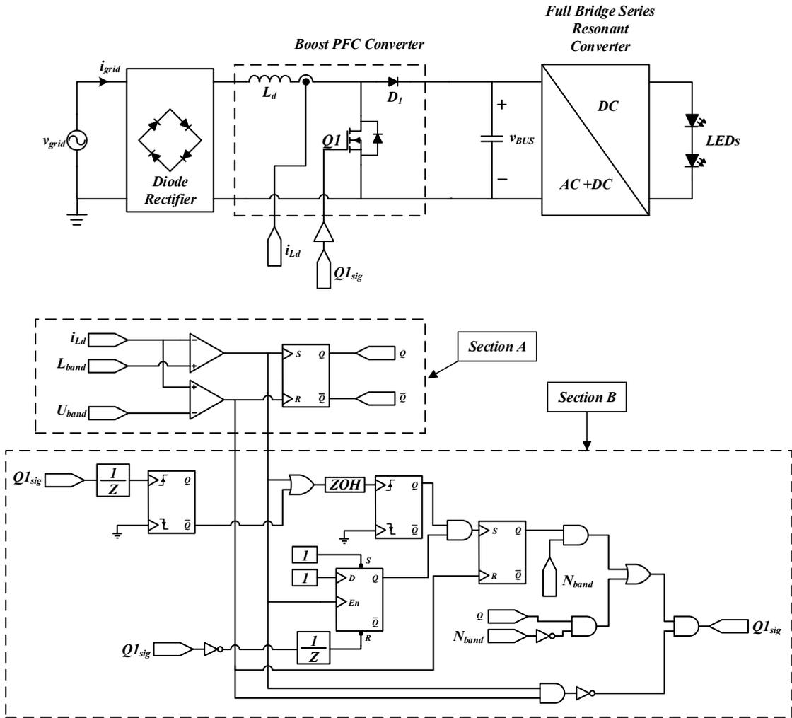
FIGURE 2.18: GPCC logic circuit
