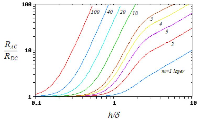
FIGURE 5.10:  $\frac{R_{AC}}{R_{DC}}$  ratio for different number of layers and frequencies
