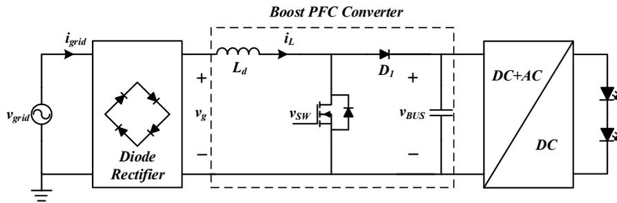
FIGURE 2.14: Step up PFC converter
