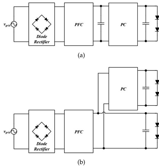
FIGURE 3.3: Multi-stage LED Driver Topologies; (a) Independent cascade structure, (b) Optimized cascade structure (RRPP)
