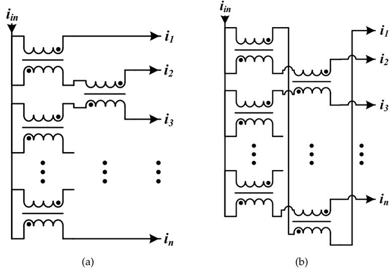
FIGURE A.9: (a) Open-Chain Transformer and (b) Daisy-Chain Transformer
