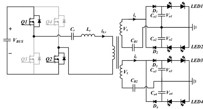
FIGURE 4.6: Mode 2 and 3 of resonant converter operation
