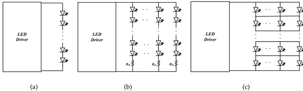
FIGURE 1.1: LED configurations;
