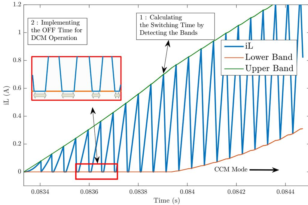
FIGURE 2.17: Band Detection and DCM OFF Time Calculation
