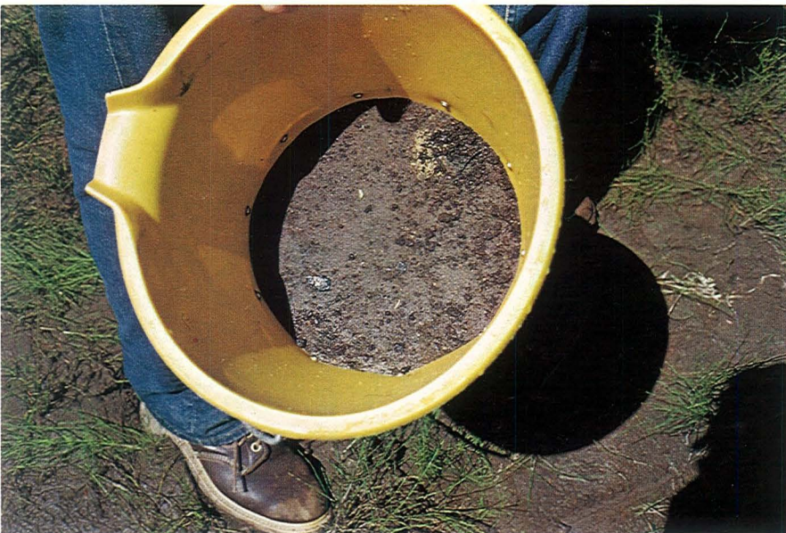
Plate 8. 23 July 1974 Wash pail for Ekman samples, containing tar sand/silt substrate from Site B1, Poplar Creek.
