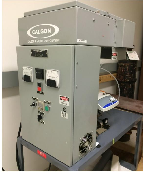
**Figure 8-1.** Medium-pressure UV lamp apparatus.
