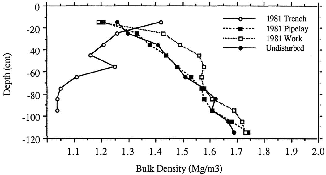
Figure 21. Site-averaged bulk density on the 1981 RoW and for the undisturbed prairie for August 1991.
