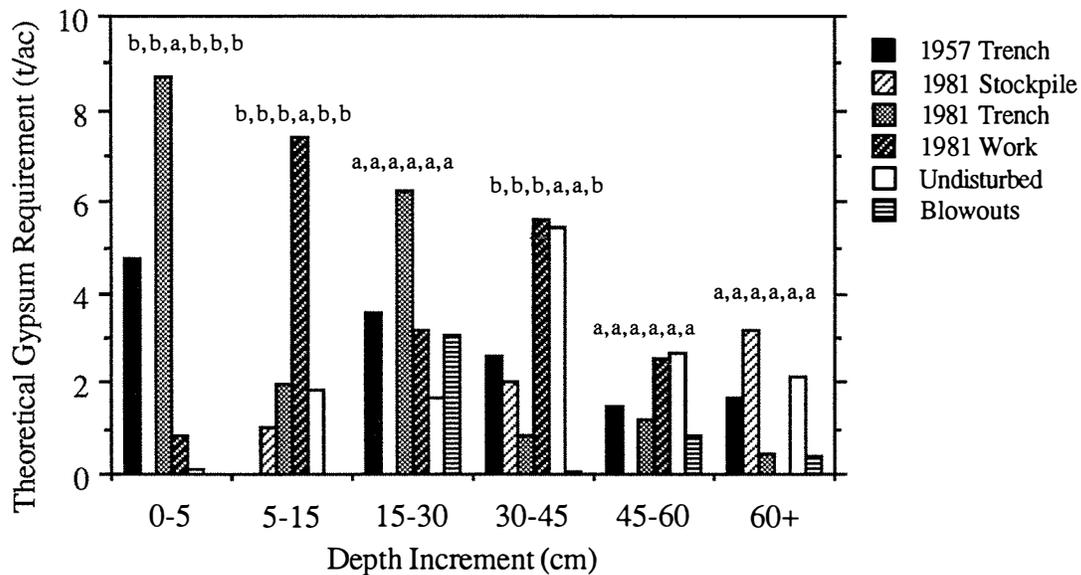
Figure 15. Theoretical gypsum requirement site-averaged profile for August 1991. Means within a given depth increment with the same letters are not significantly different at the 5% level of significance.
