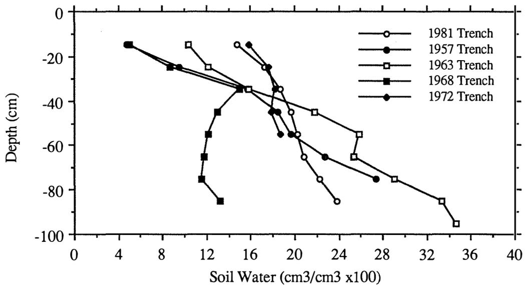
Figure 28. In-trench soil water at Site 2 for August 1991.
