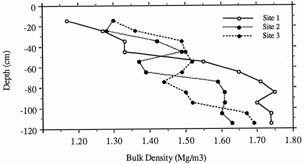
Figure 19. Bulk density in the undisturbed prairie at Sites 1, 2, and 3 for August 1991.
