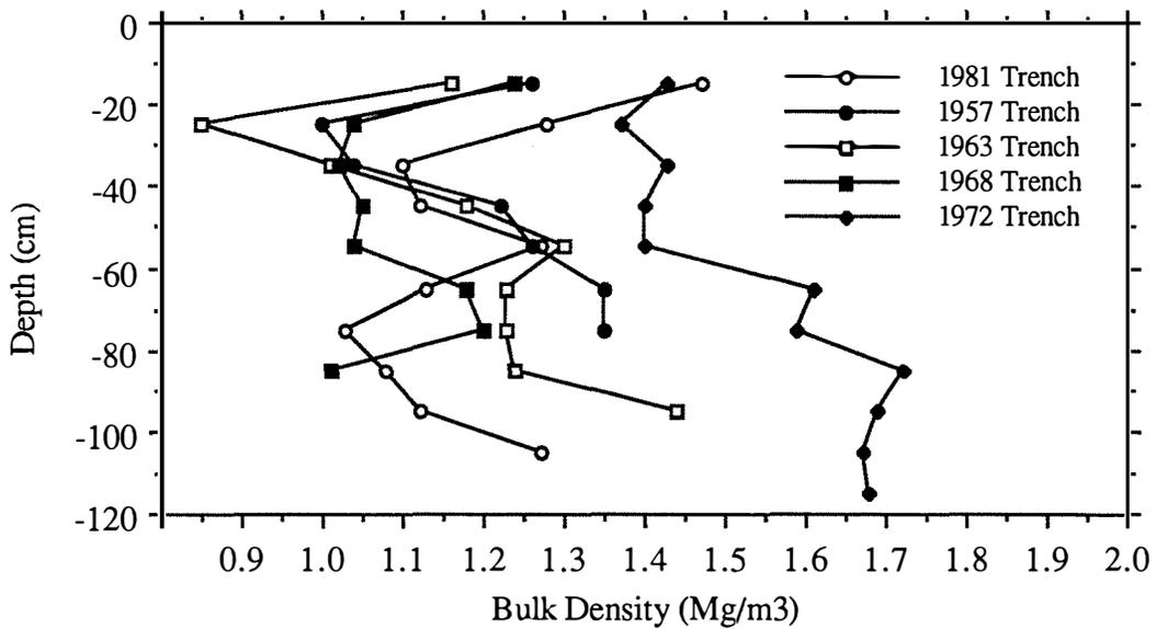
Figure 22. In-trench bulk density at Site 2 for August 1991.
