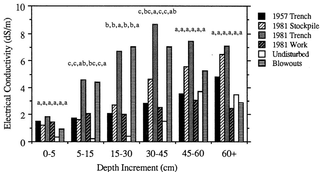
Figure 4. Electrical conductivity site-averaged profile for August 1991. Means within a given depth increment with the same letters are not significantly different at the 5% level of significance.
