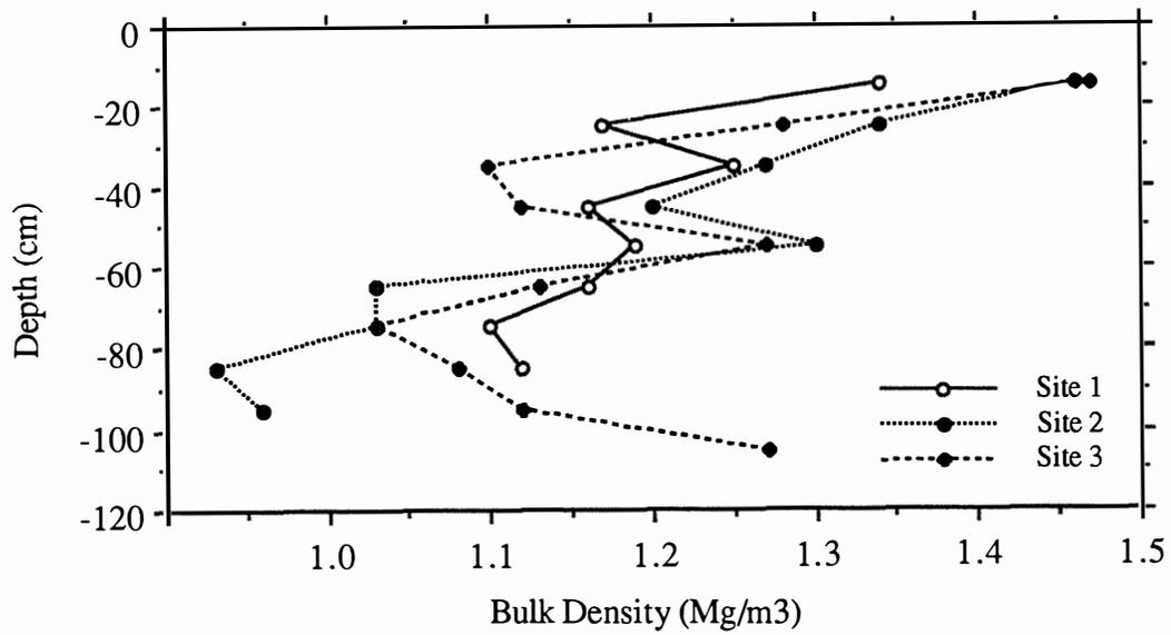
Figure 20. In-trench bulk density at Sites 1, 2, and 3 for August 1991.
