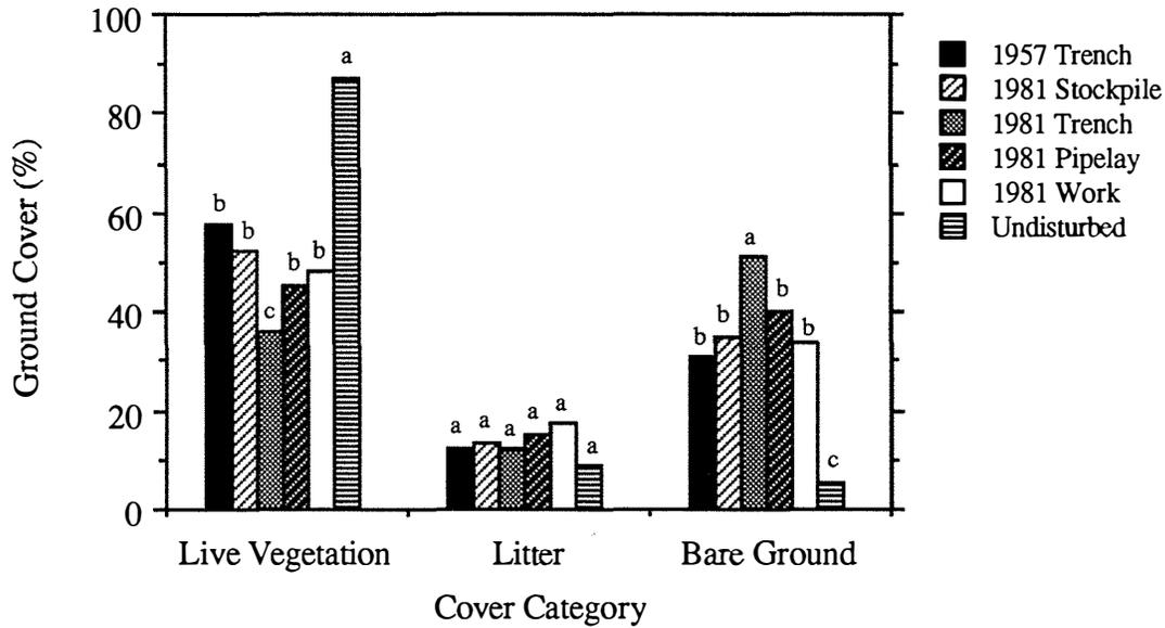
Figure 29. Site-averaged ground cover for August 1991. Means within a given vegetation type with the same letters are not significantly different at the 5% level of significance.
