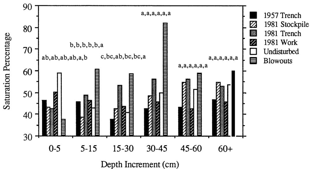
Figure 3. Saturation percentage site-averaged profile for August 1991. Means within a given depth increment with the same letters are not significantly different at the 5% level of significance.
