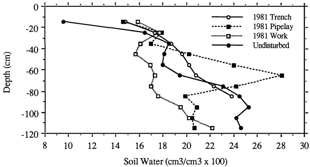
Figure 27. Site-averaged soil water on the 1981 RoW and in the undisturbed prairie for August 1991.
