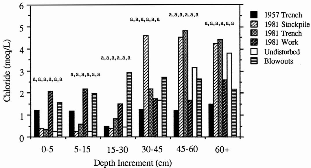
Figure 10. Chloride site-averaged profile for August 1991. Means within a given depth increment with the same letters are not significantly different at the 5% level of significance.
