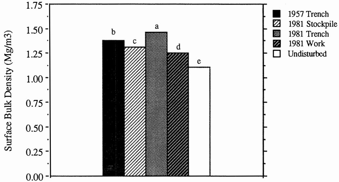
Figure 18. Site-averaged surface bulk density for August 1991. Means with the same letters are not significantly different at the 5% level of significance.
