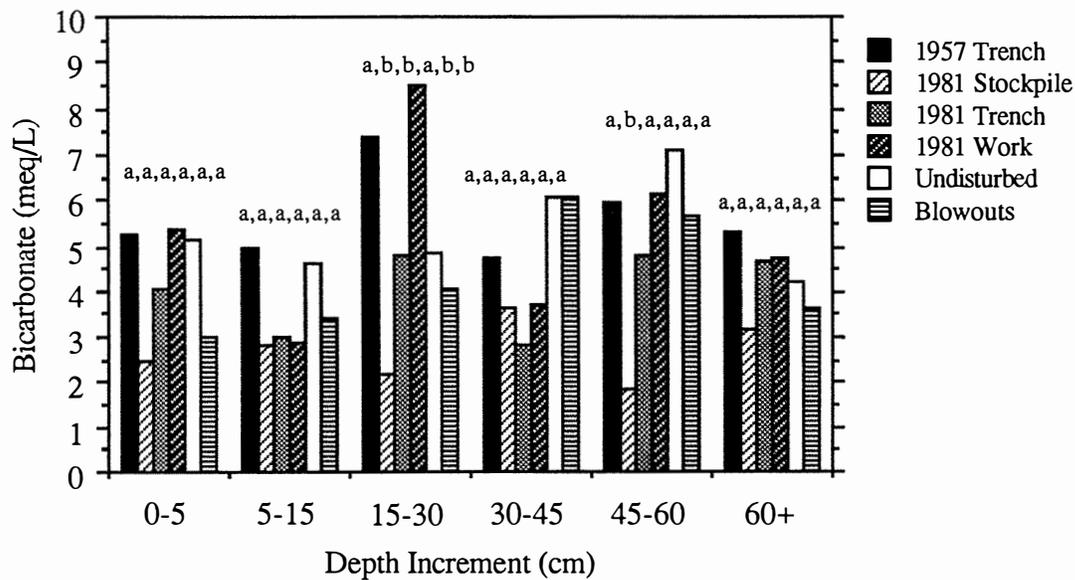
Figure 11. Bicarbonate site-averaged profile for August 1991. Means within a given depth increment with the same letters are not significantly different at the 5% level of significance.
