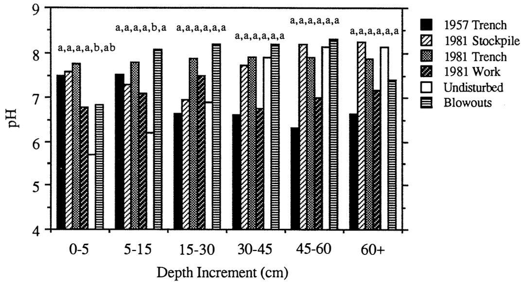
Figure 2. Soil pH site-averaged profile for August 1991. Means within a given depth increment with the same letters are not significantly different at the 5% level of significance.
