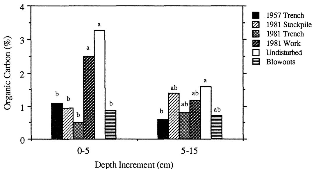
Figure 16. Organic carbon site-averaged profile for August 1991. Means within a given depth increment with the same letters are not significantly different at the 5% level of significance.
