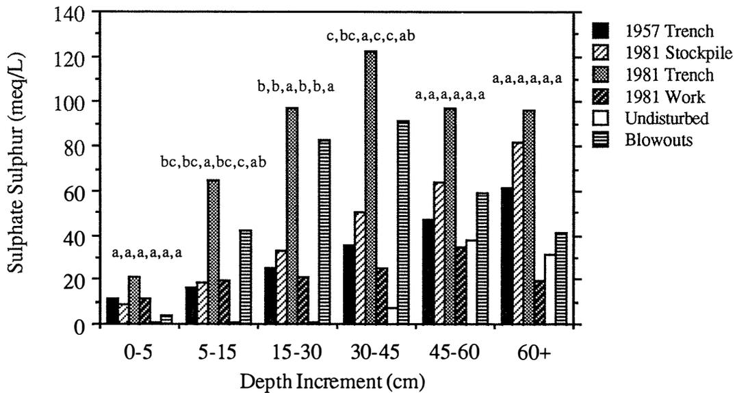
Figure 9. Sulphate sulphur site-averaged profile for August 1991. Means within a given depth increment with the same letters are not significantly different at the 5% level of significance.
