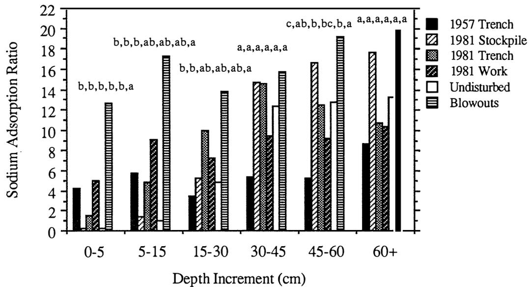
Figure 13. Sodium adsorption ratio site-averaged profile for August 1991. Means within a given depth increment with the same letters are not significantly different at the 5% level of significance.
