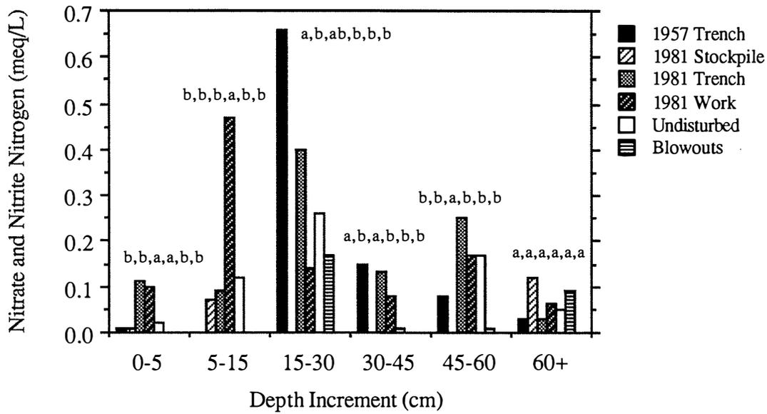
Figure 12. Nitrate and nitrite nitrogen site-averaged profile for August 1991. Means within a given depth increment with the same letters are not significantly different at the 5% level of significance.
