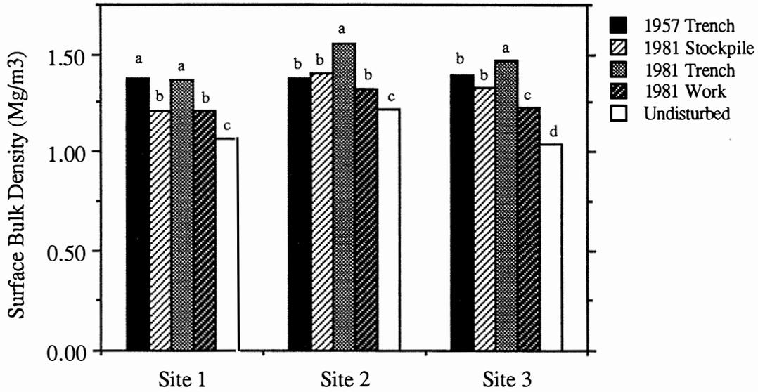
Figure 17. Surface bulk density at Sites 1, 2, and 3 for August 1991. Means within a given site with the same letters are not significantly different at the 5% level of significance.
