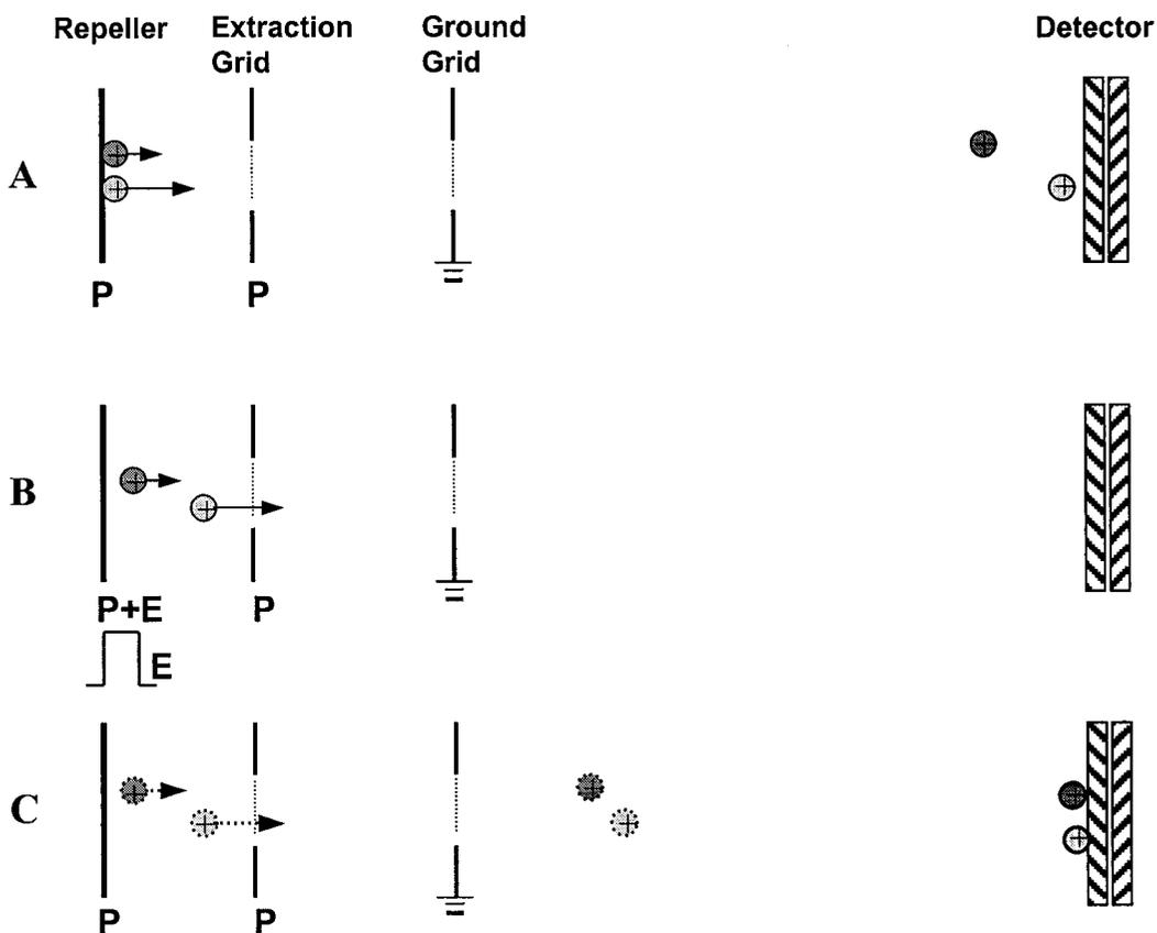
**Figure 1.4** Illustration of principle and the effect of time-lag focusing in a linear TOF MS. (A) Illustration of the flight of two ions with same  $m/z$  but different initial velocity without time-lag focusing. (B) In time-lag focusing, a pulse voltage is applied after ions are first separated by their initial velocity in the source region. (C) After the pulse voltage, the lower ion will catch up the faster one at detector.
