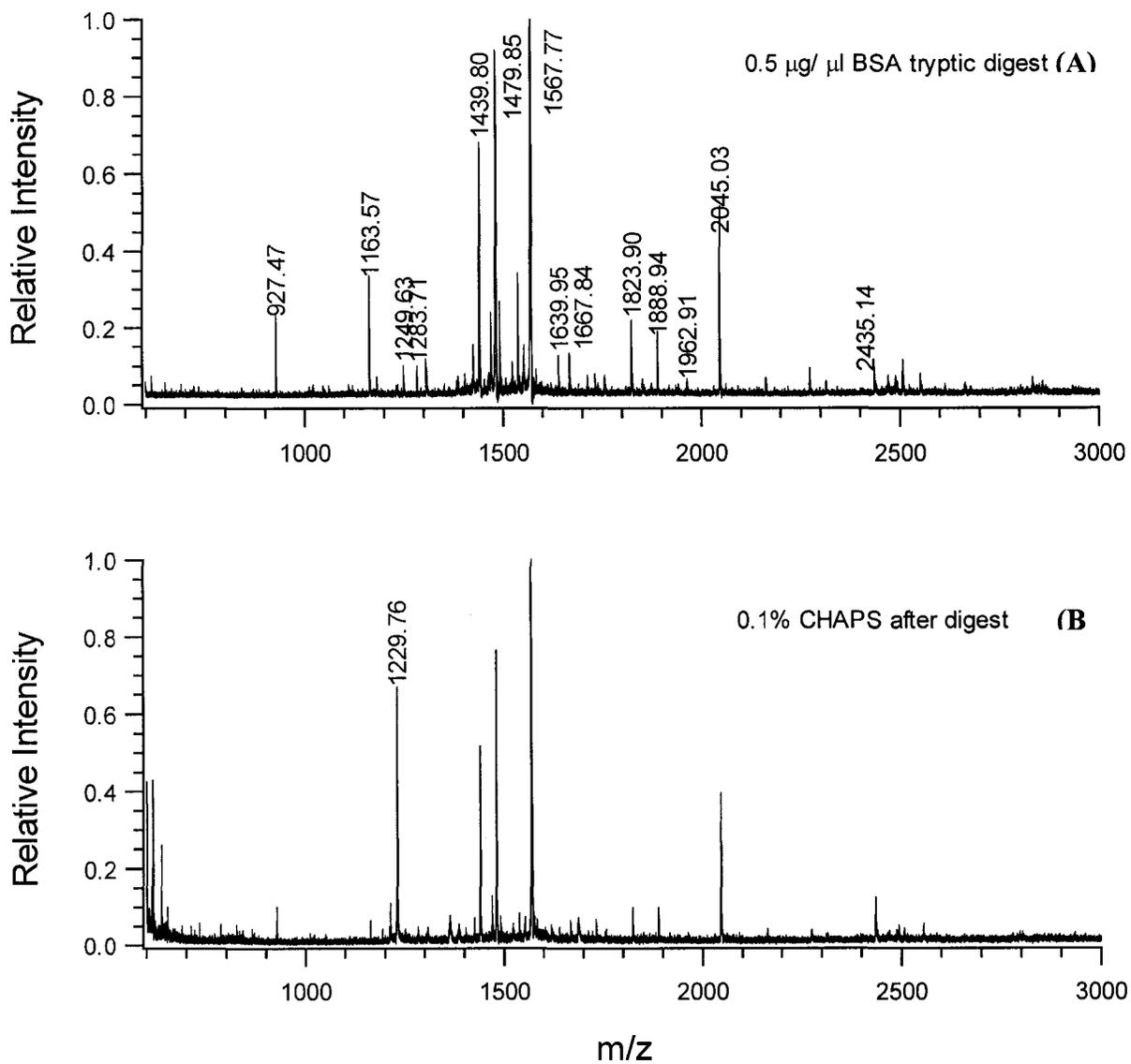
**Figure 4.2** MALDI spectra obtained from 0.5  $\mu\text{g}/\mu\text{L}$  BSA tryptic digest in (A) water and (B) add 0.1% CHAPS after digestion.
