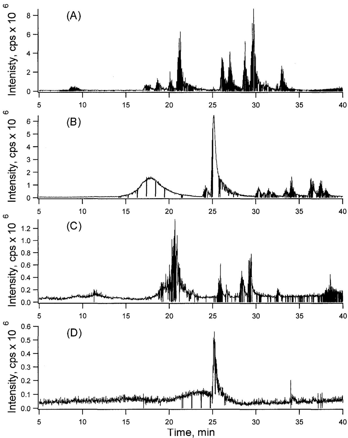
**Figure 5.5** LCQ Deca chromatograms of cytochrome c tryptic digest. (A) 8-pmol sample, (B) 8-pmol sample in 0.1% SDS with SDS removal guard column, (C) 800-fmol sample and (D) 800-fmol sample in 0.1% SDS with SDS removal guard column.
