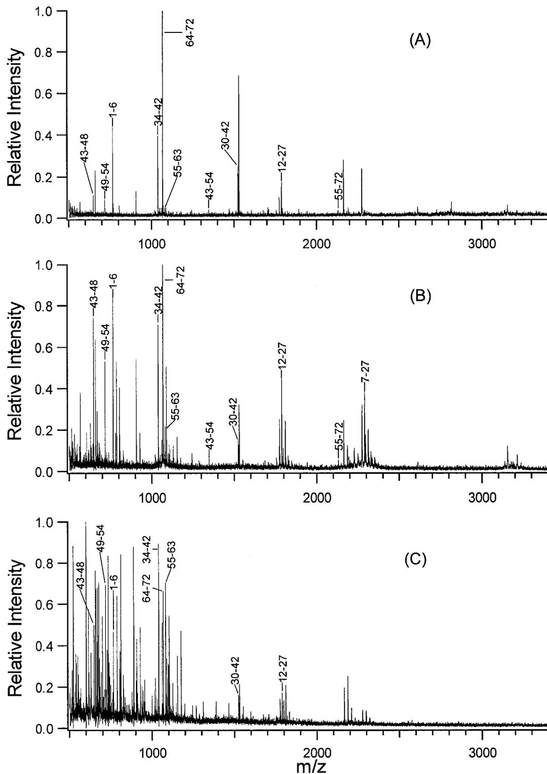
**Figure 4.6** MALDI spectra obtained from digestion of 1  $\mu\text{g}/\mu\text{L}$  ubiquitin (A) without adding SDS, (B) with 0.1% SDS added after digestion and (C) with 1% SDS added after digestion. The peptide fragments are labelled according to the amino acid sequence coverage of ubiquitin.
