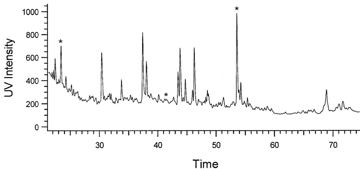
**Figure 5.2** Reversed-phase HPLC chromatogram of tryptic digest of SDS-solubilized membrane protein mixture. (The MALDI MS spectra of the fractions labeled with \* are shown in Figure 5.3)
