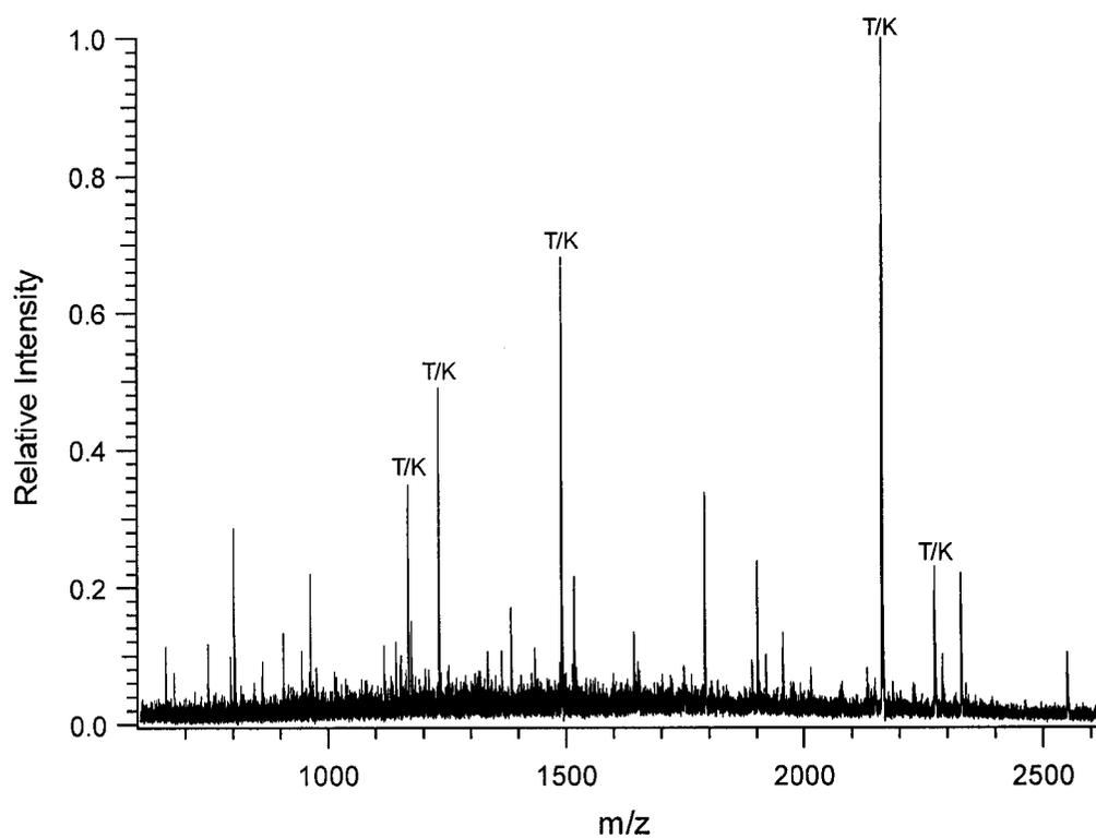
**Figure 6.1** Direct MALDI MS profiling on the SDS-containing raft digest. Digestion was efficient. However, most of the dominant peaks were from Trypsin autolysis or Keratin contamination, indicated by T/K. A limited of peptides from raft proteins were detected.
