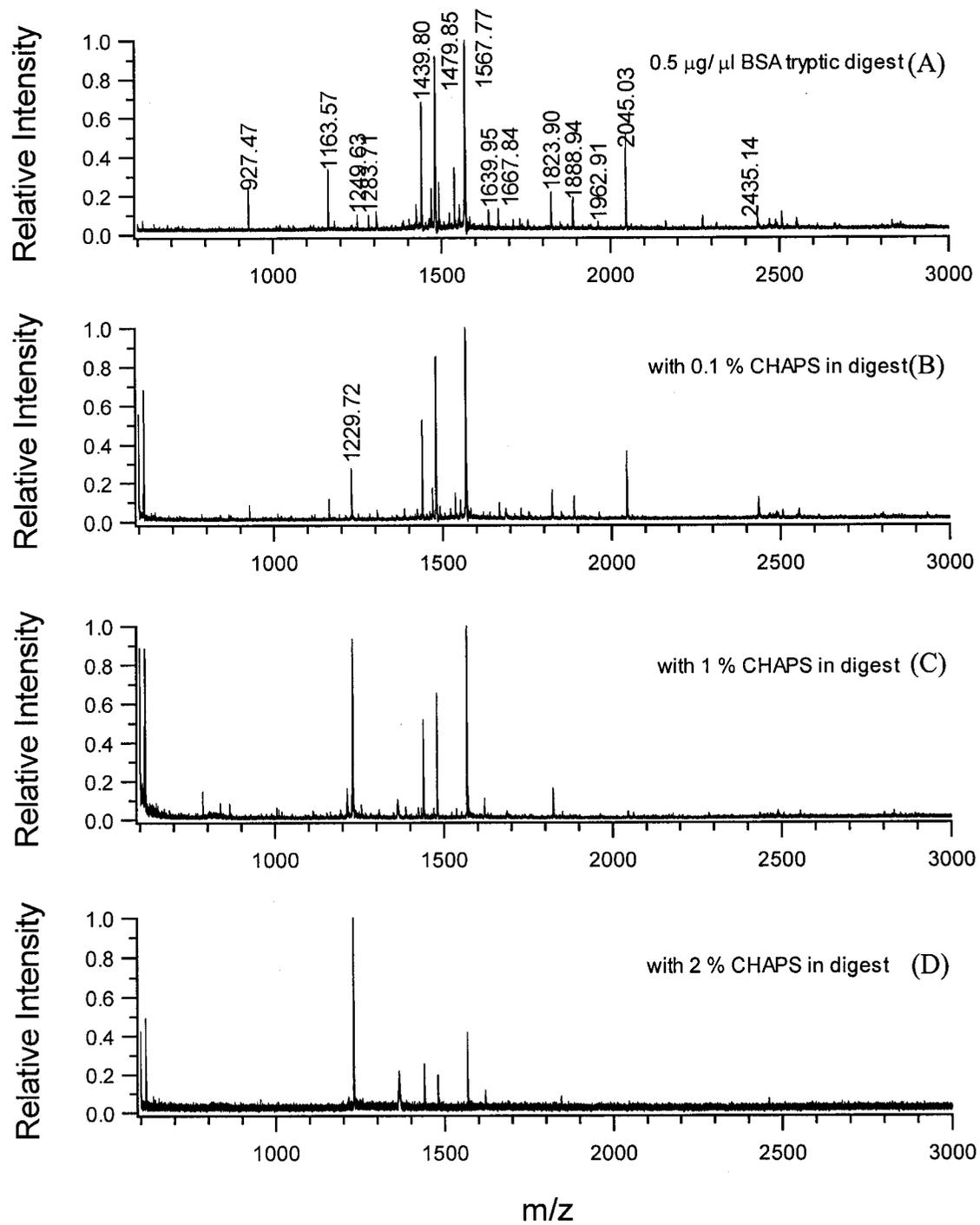
**Figure 4.1** MALDI MS spectra of 0.5  $\mu\text{g}/\mu\text{l}$  BSA digested with presence of (A) no surfactant, (B) 0.1%, (C) 1%, and (D) 2% CHAPS.
