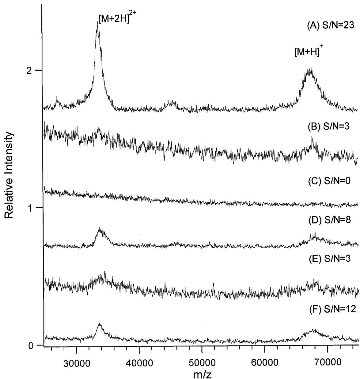
**Figure 2.1** MALDI spectra obtained from samples of 500 nM BSA prepared in (A) 0% SDS, (B) 0.05% SDS, (C) 1% SDS, without on-probe washing; and in (D) 0% SDS, (E) 0.05% SDS, (F) 1% SDS, with the addition of on-probe washing. (A) & (D), (B) & (E), and (C) & (F) were from same sample spot. The calculated signal to noise of the molecular ion peak is indicated in the figure.
