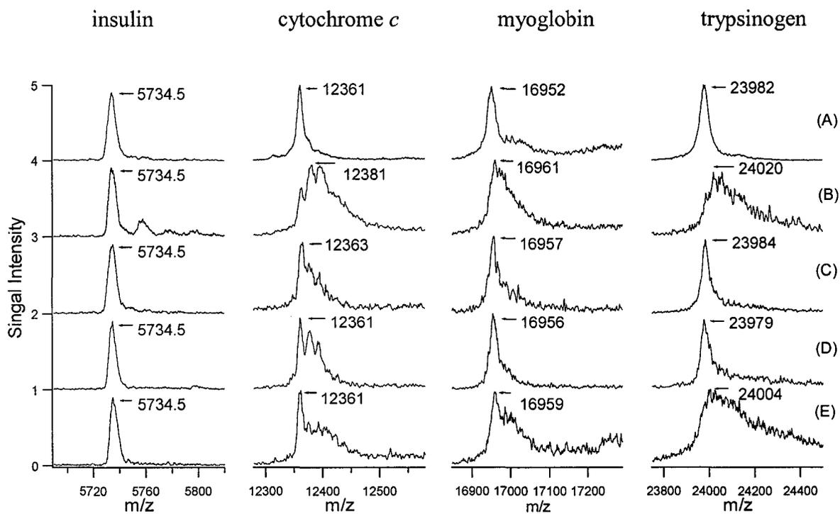
**Figure 3.2** MALDI spectra of 2  $\mu$ M insulin, cytochrome *c*, myoglobin, and trypsinogen: (A) without surfactant, (B) with 0.5% SDS, (C) with 0.5% HDS, (D) with 0.5% ADS, and (E) with 0.5% TDS. Analyte to matrix ratio varies from 1:1 to 1:2.
