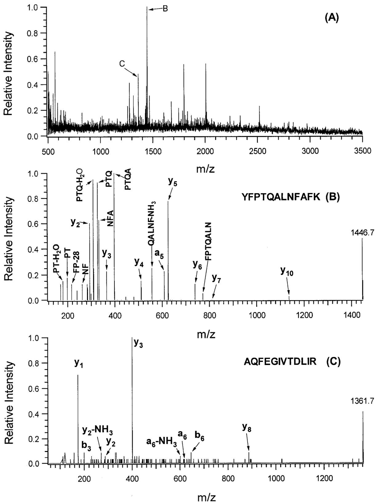
**Figure 5.4** MALDI MS spectrum of HPLC 50 min fraction (A), and MALDI MS/MS spectra of peptides 1446.6 Da (B) and 1361.7 Da (C).
