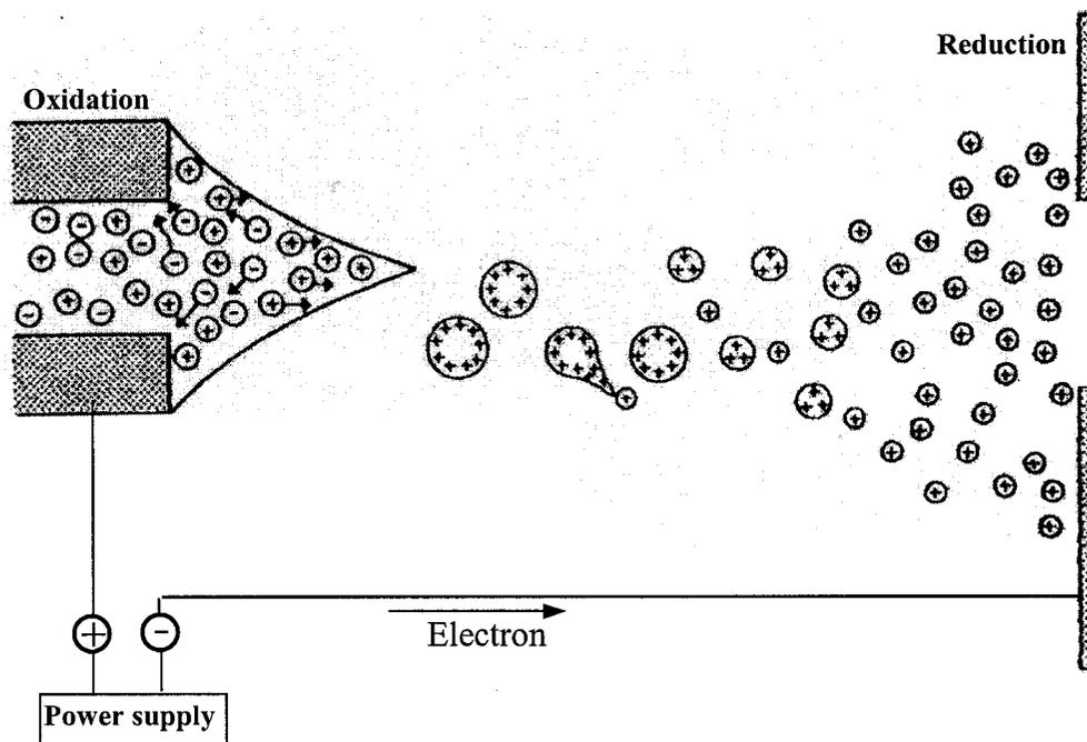
**Figure 1.6** Schematic representation of processes in ESI.
