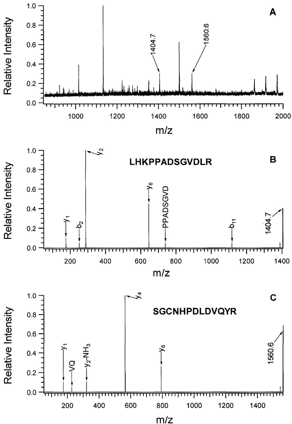
**Figure 6.3** MALDI MS spectrum of HPLC fraction 36 min (A) and sequencing patterns of peptides 1404.7 and 1560.6 (B and C). Two sequences were assigned as shown, leading to the identifications of protein monocarboxylate transporter 4, O15427, and urokinase plasminogen activator surface receptor, GPI-anchored form, Q03405, respectively.
