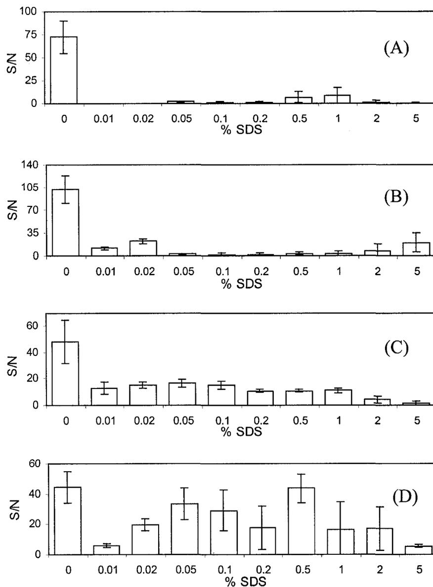
**Figure 2.2** Average signal to noise ratios (S/N) for the molecular ion signals calculated from the MALDI spectra of 1  $\mu$ M cytochrome *c* at various concentrations of SDS. The matrices used for the analysis are (A) sinapinic acid, (B) HCCA, (C) HABA, (D) DHB. Error bars represent the standard deviations of S/N from 9 spectra recorded from 3 independent sample spots (A, C, D) or 3 independent spectra (B).
