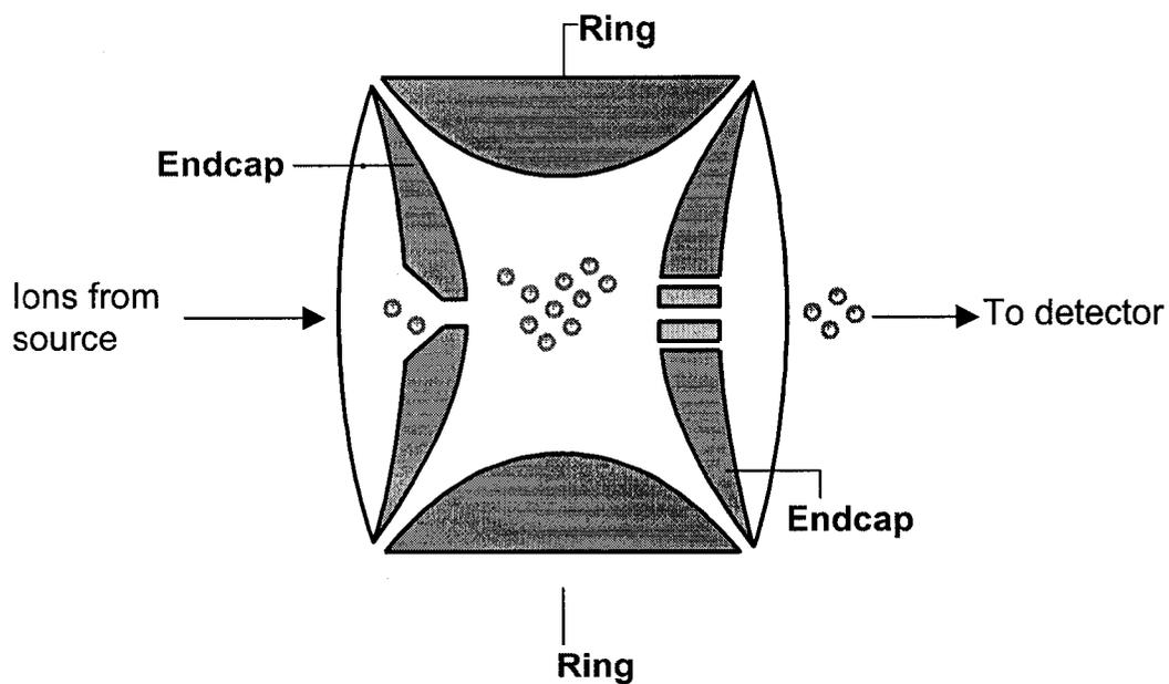
**Figure 1.8** Schematic diagram of ion trap mass analyzer.
