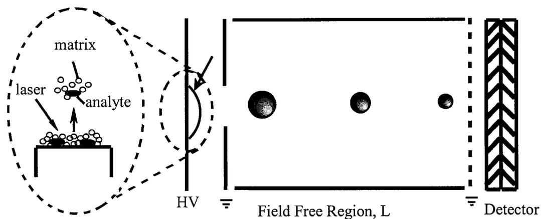
**Figure 1.3** Schematic graph of a linear MALDI-TOF mass spectrometer.
