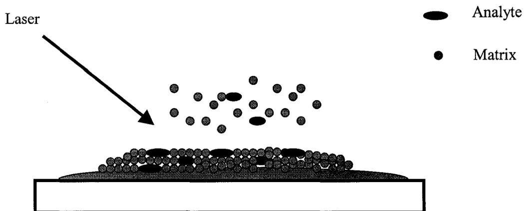
**Figure 1.1** Schematic diagram of MALDI.
