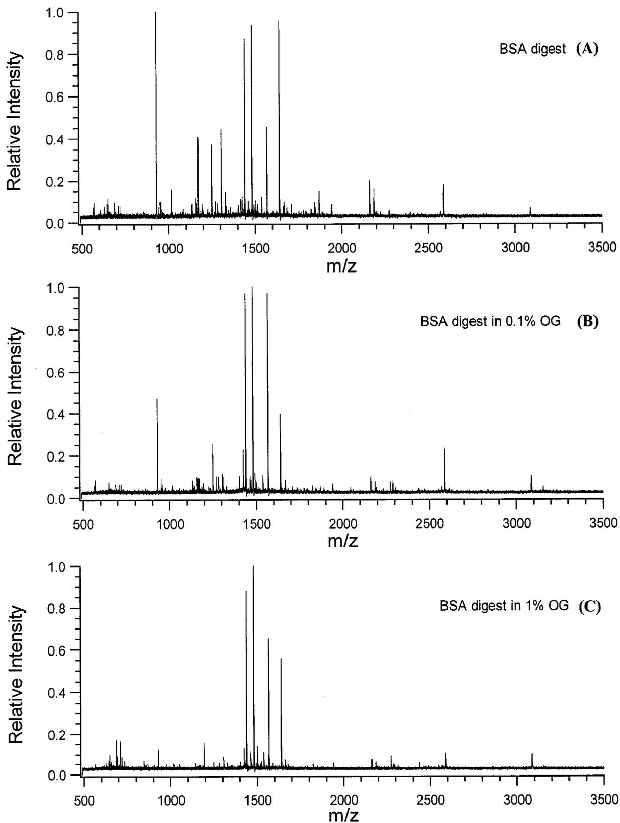
**Figure 4.4** MALDI MS spectra of 0.5  $\mu\text{g}/\mu\text{l}$  BSA digested with the presence of (A) no surfactant, (B) 0.1%, (C) 1% OG.
