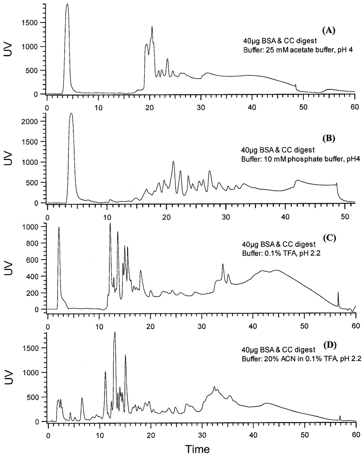
**Figure 7.1** Chromatograms of the cation exchange separation of 40 µg BSA and cytochrome c tryptic digest under different mobile phase buffers. Solvents: A is buffer indicated in the graph; B is 0.5M NaCl in A.
