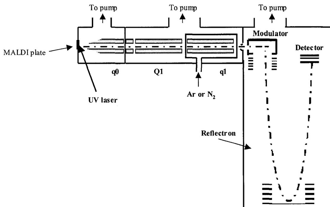
**Figure 1.9** Schematic diagram of a hybrid quadrupole time-of-flight mass spectrometer.
