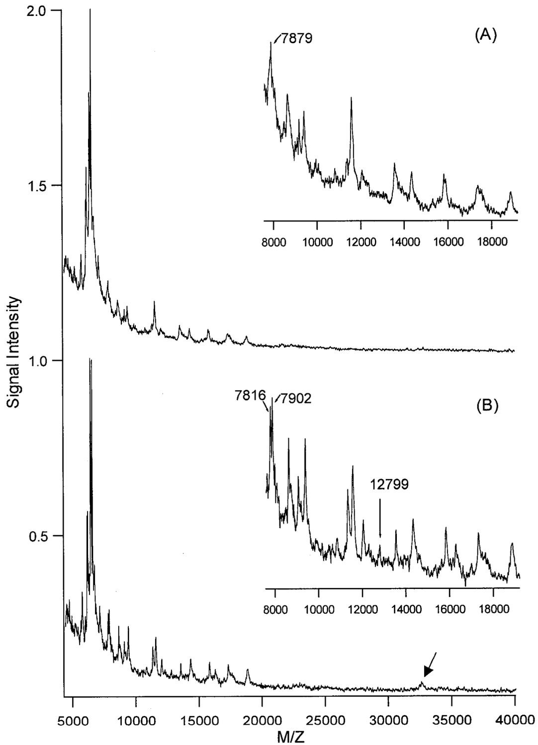
**Figure 3.5** MALDI spectra of the CD9 cell lysate Detergent Insoluble Fraction pellet. The pellet was mixed with (A) 1% SDS and (B) 1% ADS.
