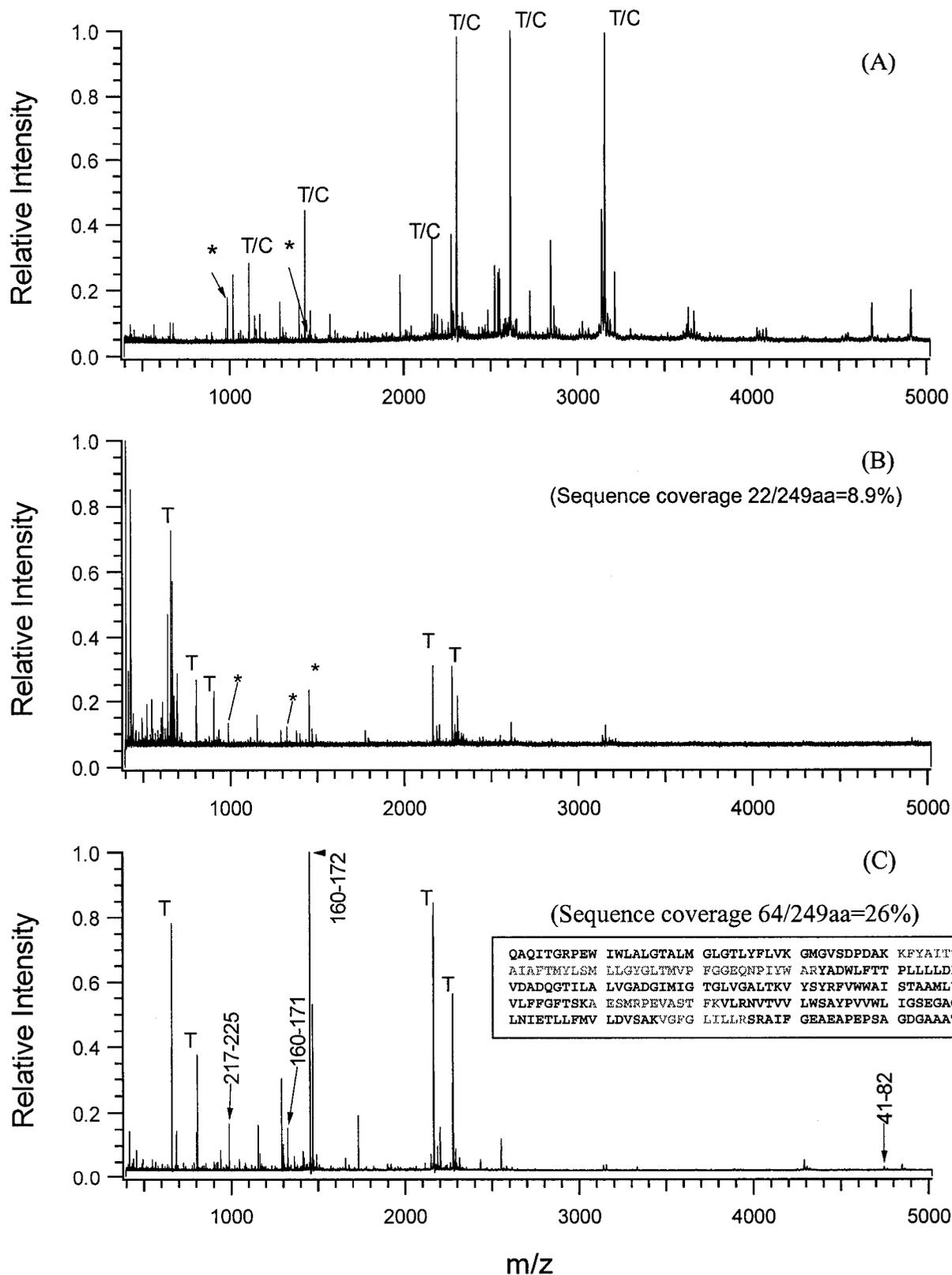
**Figure 4.8** MALDI MS spectra of BRO tryptic digestion with (A) no SDS, (B) 0.1% SDS added after digestion and (C) 0.1% SDS present during digestion. (T/C indicates trypsin autolysis or commonly observed peaks in gel analysis.)
