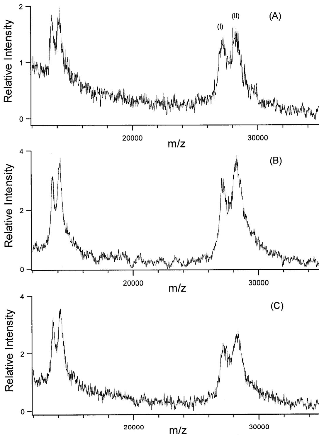
**Figure 2.5** MALDI spectra obtained from samples of 0.25  $\mu\text{g}/\mu\text{L}$  bacteriorhodopsin with (A) 0% SDS, (B) 0.1% SDS and (C) 1% SDS using HCCA matrix and a two-layer deposition method. The labeled peak I indicates the bacteriorhodopsin molecular ion signal and the peak labeled as II is likely from an unprocessed precursor of bacteriorhodopsin.
