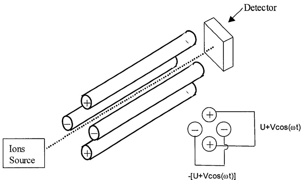
**Figure 1.7** Schematic representation of the quadrupole mass filter and basic principle.
