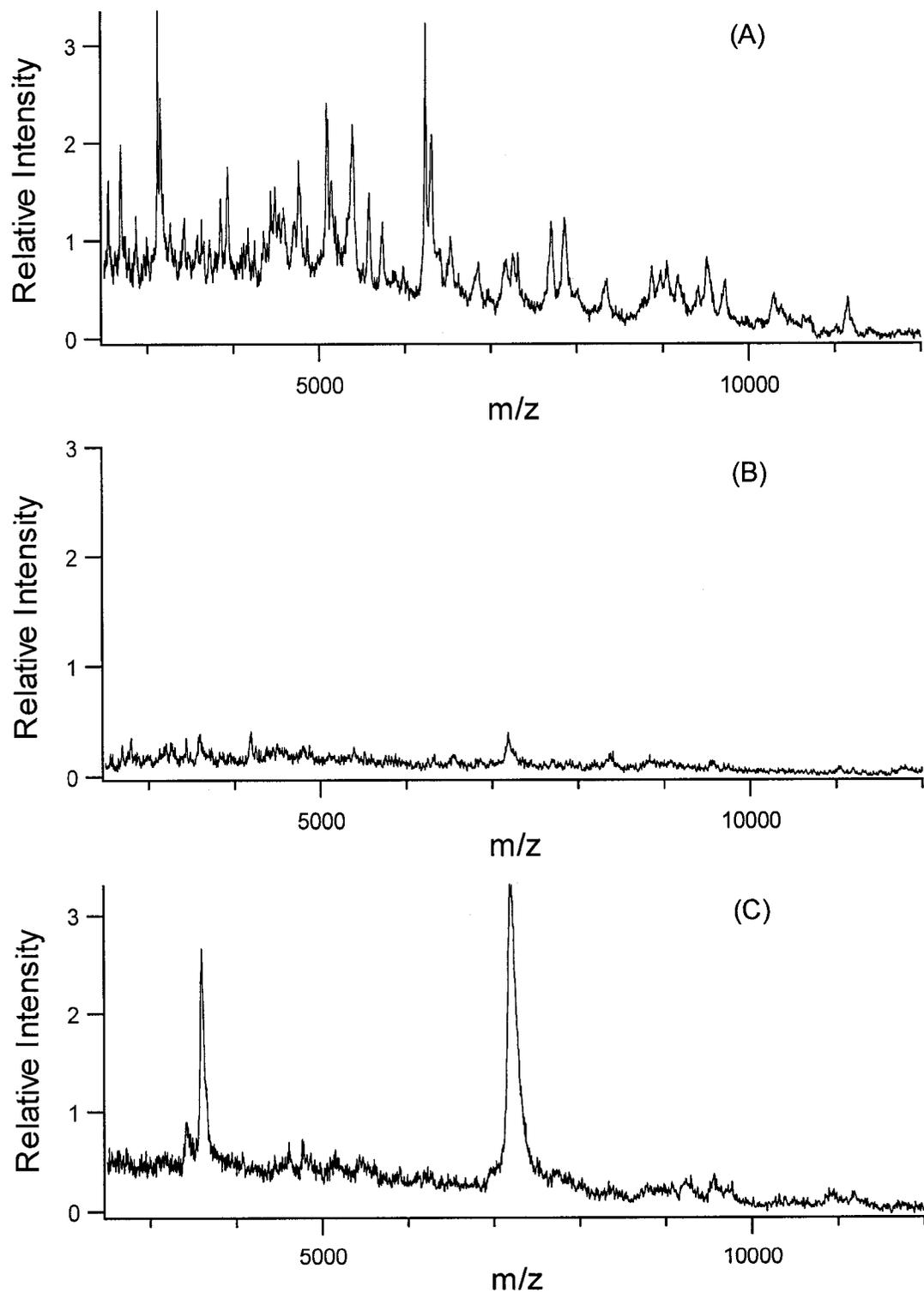
**Figure 2.6** MALDI spectra obtained from sequential extractions of an *E. coli* sample: (A) first extract with 0.1% aqueous TFA, (B) second extract with 0.1% aqueous TFA, and (C) third extract with 0.2% SDS in 0.1% TFA.
