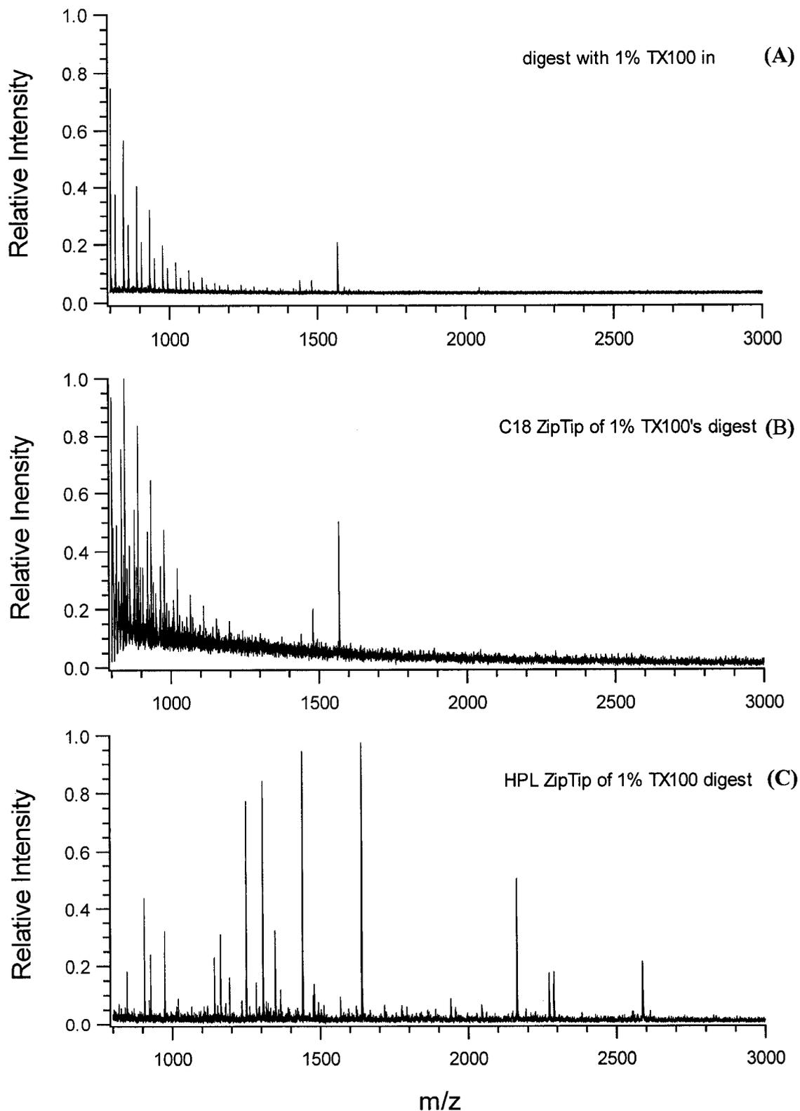
**Figure 4.3** MALDI spectra of 0.1  $\mu\text{g}/\mu\text{L}$  BSA tryptic digestion with 1% Triton X 100 (A), (B) after C<sub>18</sub> ZipTip cleanup, and (C) after HPL ZipTip cleanup.
