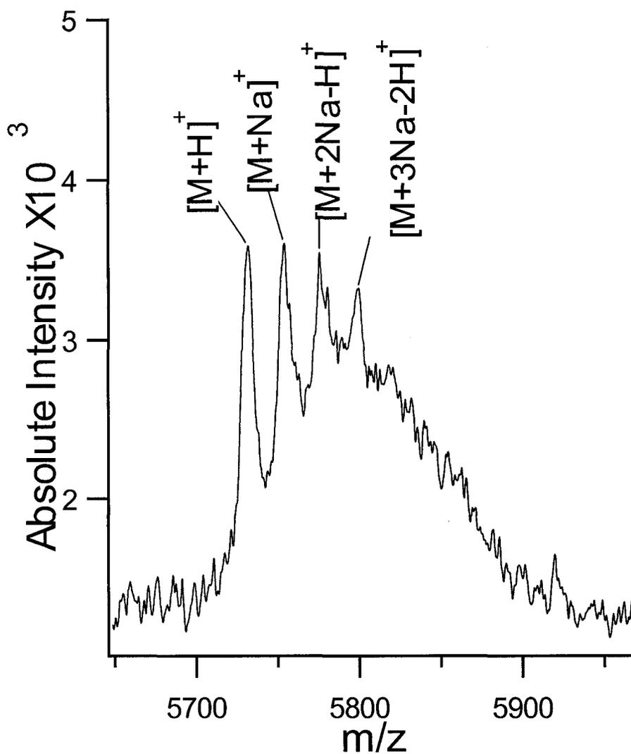
**Figure 3.1** MALDI spectrum of 2  $\mu$ M bovine insulin with 2% SDS. Analyte to matrix, HCCA (saturated in 40% MeOH/H<sub>2</sub>O), ratio is 1:1.
