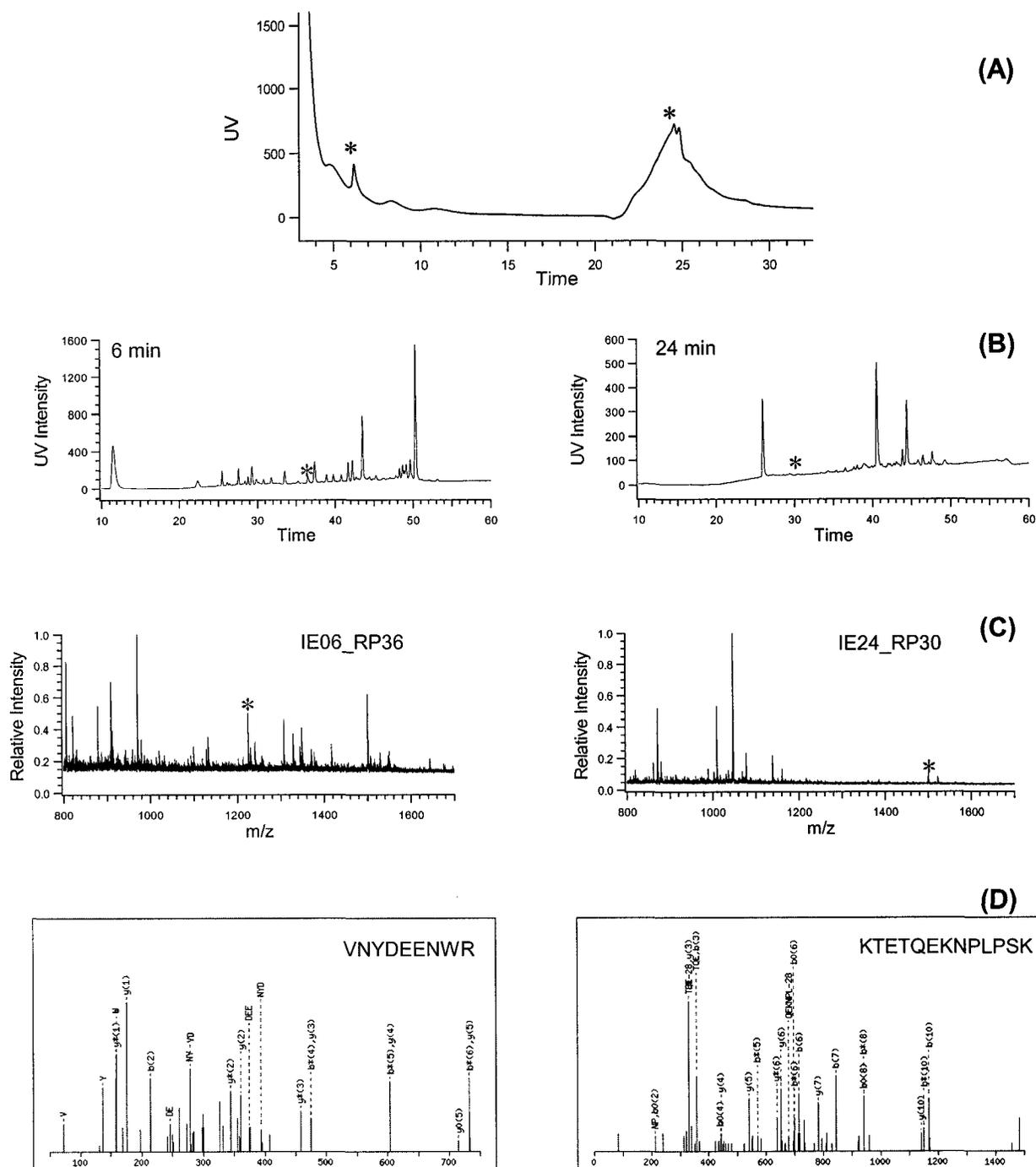
**Figure 7.4** 2D LC-MALDI MS/MS analysis of lipid raft. (A) UV chromatogram of ion exchange (IE) separation. (B) UV chromatograms of reversed-phase (RP) separation of IE fractions 06min and 24 min respectively. (C) MALDI MS spectra of RP fractions indicated in B. (D) MALDI MS/MS spectra from the peptides labeled in C with best database matches.
