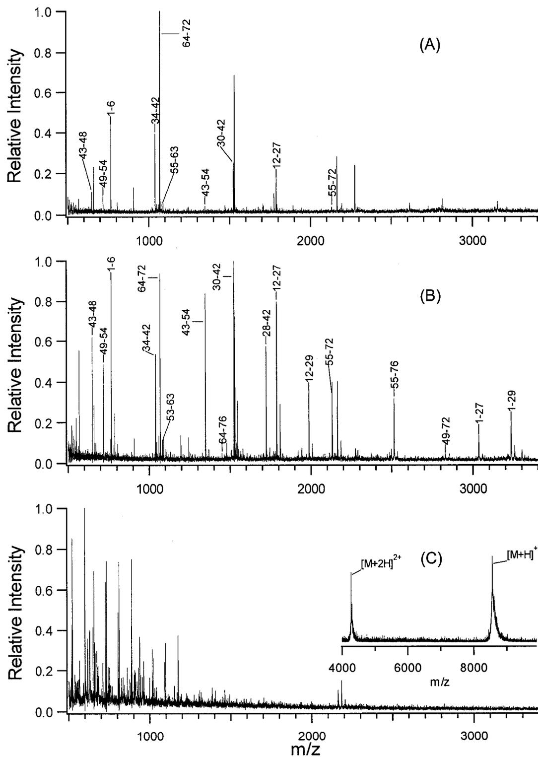
**Figure 4.7** MALDI spectra obtained from digestion of 1  $\mu\text{g}/\mu\text{L}$  ubiquitin (A) without adding SDS, (B) with 0.1% SDS added prior to digestion and (C) with 1% SDS added prior to digestion. The peptide fragments are labelled according to the amino acid sequence coverage of ubiquitin.
