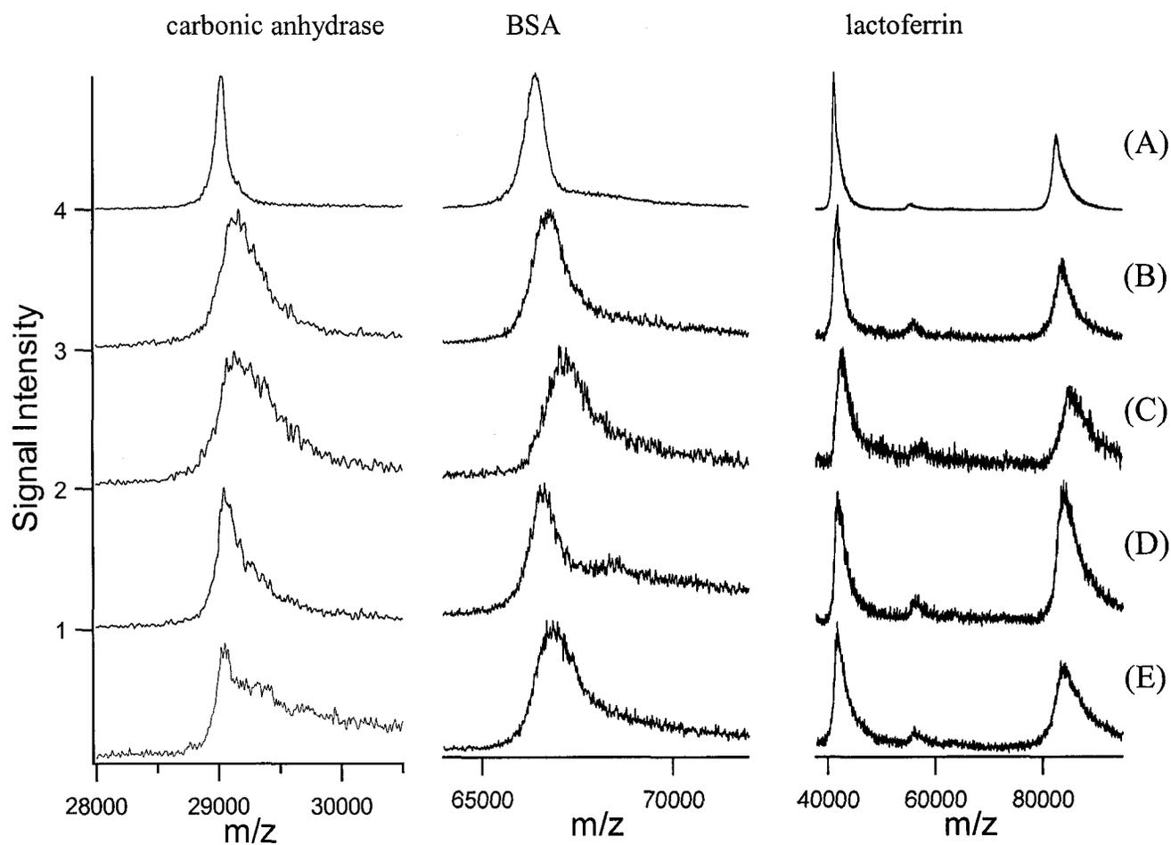
**Figure 3.3** MALDI spectra of 5  $\mu$ M carbonic anhydrase, BSA and lactoferrin: (A) without surfactant, (B) with 0.5% SDS, (C) with 0.5% HDS, (D) with 0.5% ADS, and (E) with 0.5% TDS. Analyte to matrix ratio varies from 1:1 to 1:2.
