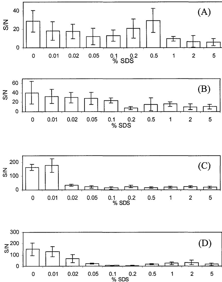
**Figure 2.4** Average signal to noise ratios (S/N) for the molecular ion signals obtained from the MALDI spectra of BSA at various concentrations of SDS. (A) 500 nM, (B) 1.5  $\mu$ M, (C) 5  $\mu$ M, or (D) 15  $\mu$ M BSA was mixed with the second-layer matrix solution in a ratio of 1:4. The second-layer matrix solution consisted of 40% methanol/water HCCA matrix. Error bars represent the standard deviations of S/N from 3 independent spectra.
