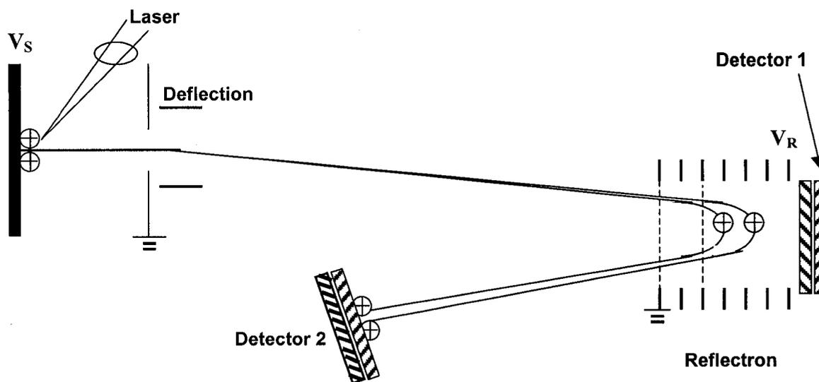
**Figure 1.5** Schematic diagram of a reflectron TOF mass spectrometer.  $V_s$  represents the voltage applied to repeller, and  $V_R$  represents the voltage grid applied on the reflectron.
