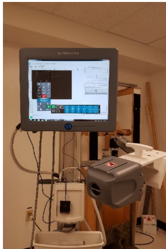
Figure 2. The ultrasound machine comprised of the SonixTABLET system and SonixGPS system.
