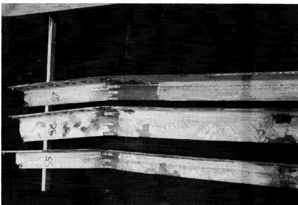
Figure 4.1 Deformed Single Angles
