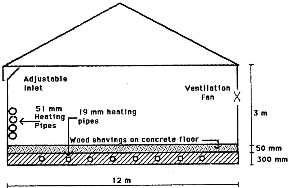
Figure 4.2 Cross-sectional view of the brooder barn showing heating pipes and inlet location (not to scale).
