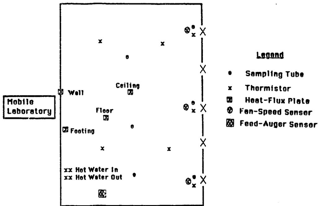
Figure 4.3 Locations of sampling, tubes and sensors in brooder barn.
