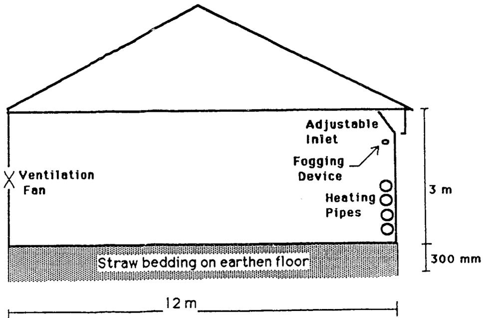
Figure 4.4 Cross-sectional view of the grower barn showing heating pipes and inlet location (not to scale).
