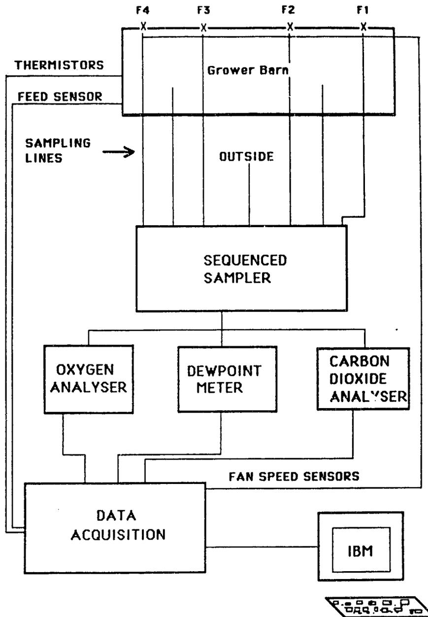
Figure 4.6 Sampling, analysing and data acquisition system in the grower barn.
