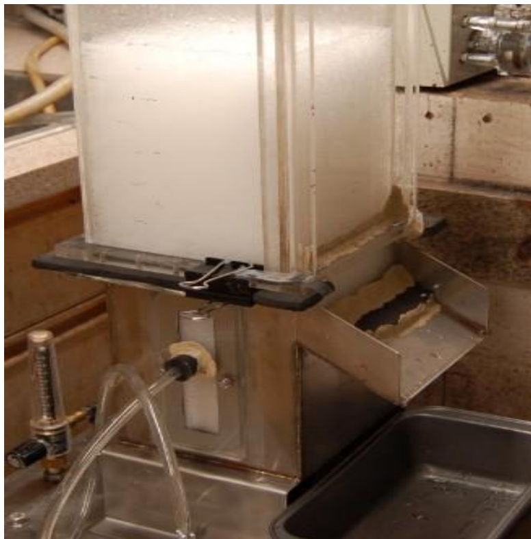
Figure 4.3 Outlet for controlling the level of pulp/froth interface
