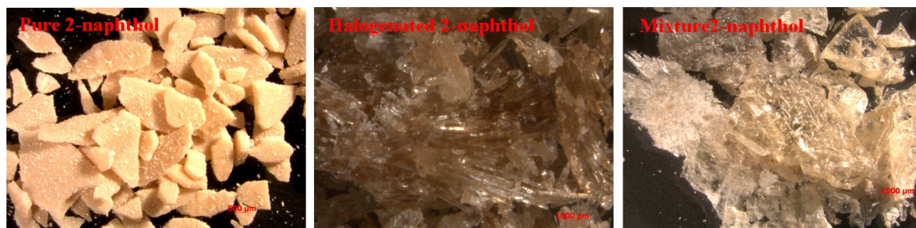
Figure 4.19. Zeiss microscopy analysis pure 2-naphthol, halogenated 2-naphthol and mixture of halogenated and pure 2-naphthol
