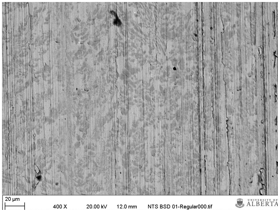
Figure 4.11 - SEM image of carbides on a sample coupon. Carbides represented by darker grey shaded areas
