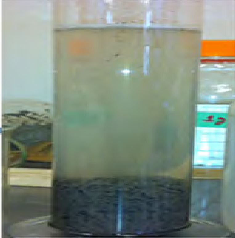
Photograph 3-21: Settling test performed on the geo-composite recipe (treated FFT with fibers).
