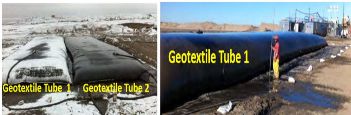
Photograph 4-8: Field trial to evaluate dewatering of the treated FFT discharged into geotextile tubes, including solids and water mass balance (section 4.1.3).
