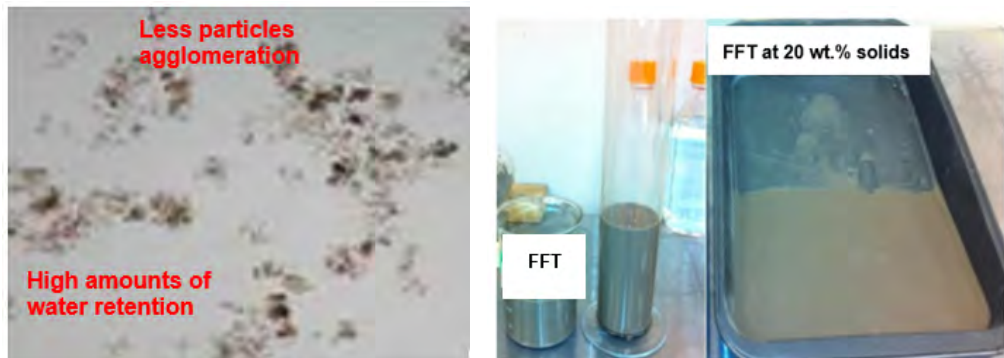
Figure 1-4: Schematic example of poor flocculation (particle dispersion and water retention).
