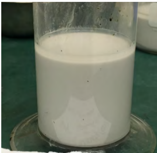
Photograph 3-7: Mixture of quartz particles (55 wt.%) + kaolinite particles (45 wt.%) + 72 ppm \text{Ca}^{2+} ions to form a suspension at 15 wt.% solids.
