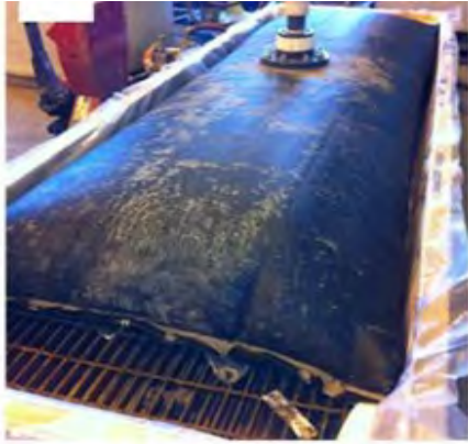
Photograph 3-14: FFT with flocculant only at 8 wt.% solids discharged into a geotextile tube. No water was released, and the tube behaved as a waterbed-like mattress during several months after filling.
